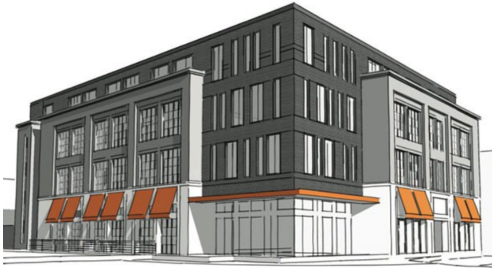
Example of a Mixed-Use Building with a Taller First Floor Ceiling Height
