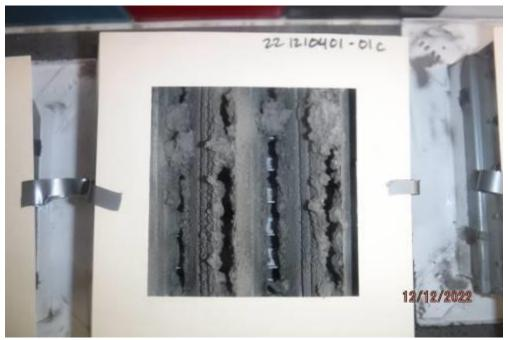
The main level all gender restroom exhaust duct vent interiors contained meth in excess of the decontamination criteria.
