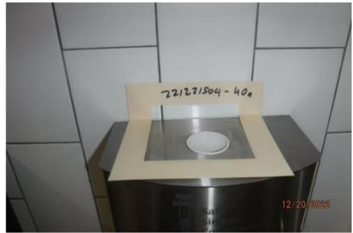
The main level all gender bathroom contact surfaces contained meth in excess of the decontamination criteria.
