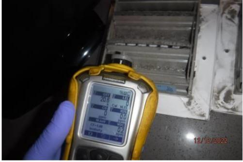
The north building women's restroom exhaust duct and contact surfaces contained no amplified TVOC concentrations, but did identify meth in excess of the decontamination criteria.
