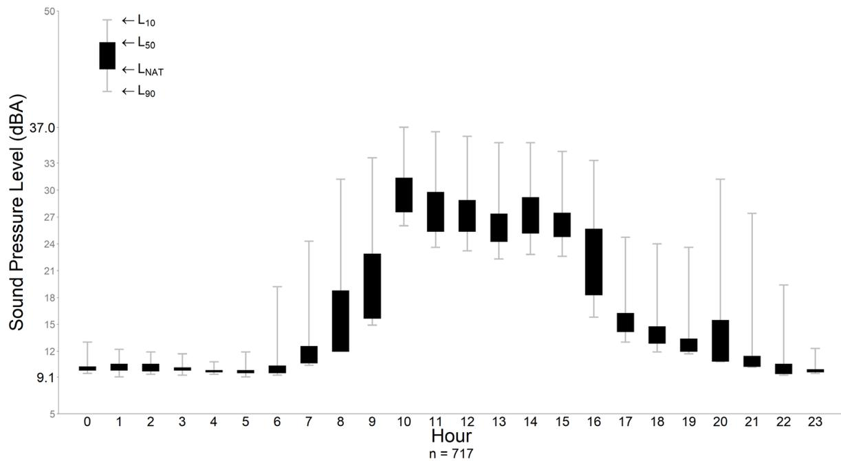
Figure 4. Median percentile sound levels ( $L_{Aeq, 1s}$ ), in dB re 20  $\mu$ Pa (Standard sound pressure reference level), at Aspen001 during the fall.
