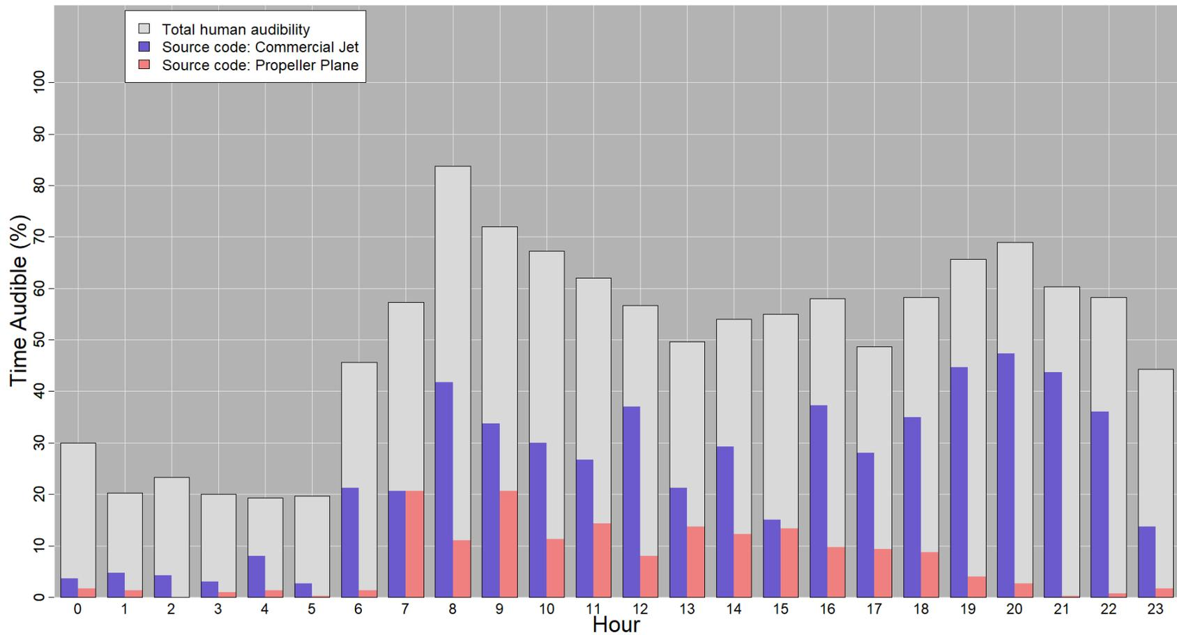
Figure 6. Hourly time audibility for commercial jets, propeller planes, and all noise sources at Aspen001 during the fall.
