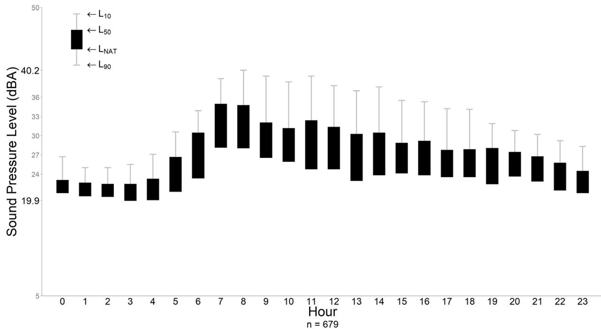
Figure 5. Median percentile sound levels ( $L_{Aeq, 1s}$ ), in dB re 20  $\mu$ Pa (Standard sound pressure reference level), at Whiterocks001 during the fall.
