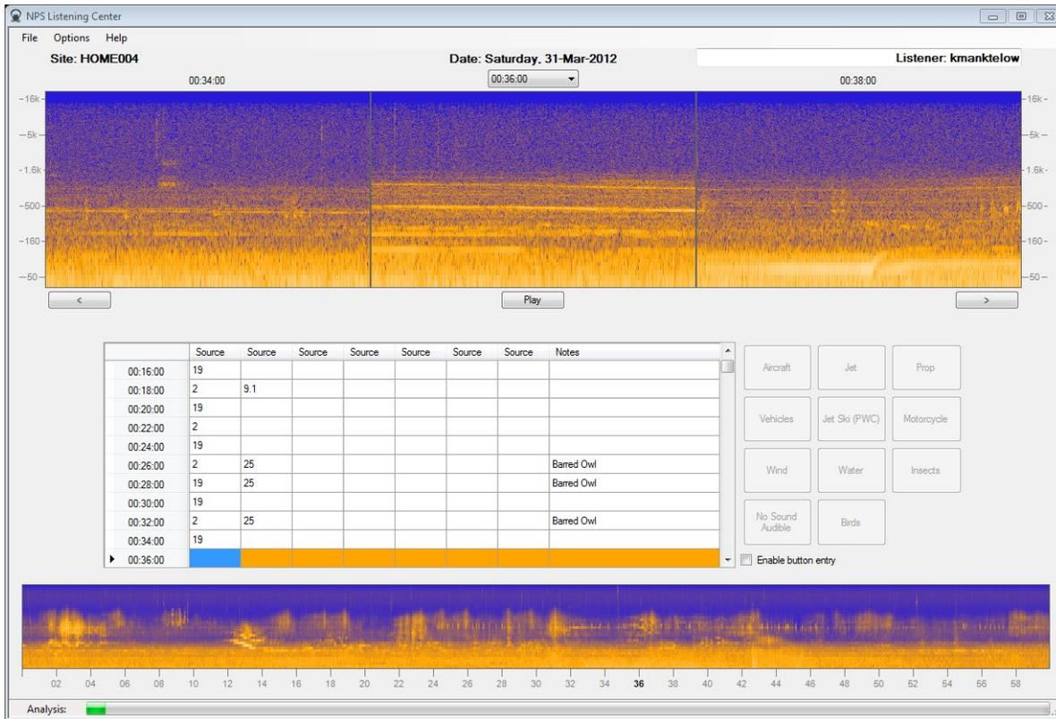
Figure 2. Screen shot of Listening Center. Three ten second samples are displayed side by side. Audible sound sources and annotations are recorded in the spreadsheet cells below.
