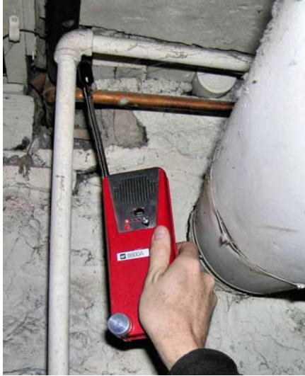
Figure 2-9. Combustion gas sniffer at work.
