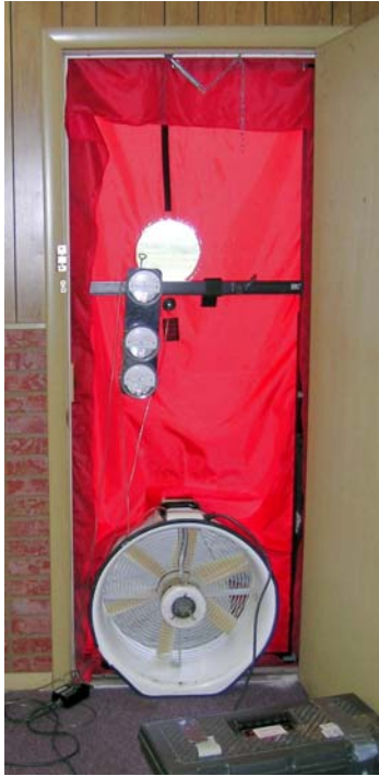
Figure 2-1. The blower door can be set up in a variety of doorways. The meters allow for measuring flow versus pressure difference as the fan speed is varied. The results can help estimate the magnitude of convective losses over a heating season. The heating bill to offset convective losses in some homes in Boulder's historic district exceed $500 per winter.
