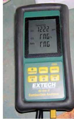
Figure 2-10. Combustion analyzer capable of measuring five functions. This one found a surprisingly high carbon monoxide reading associated with the broiler in a modern, high-end cooking stove.
