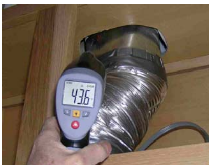
Figure 2-2. Infrared (IR) sensors like this one measure surface temperatures at a distance.
