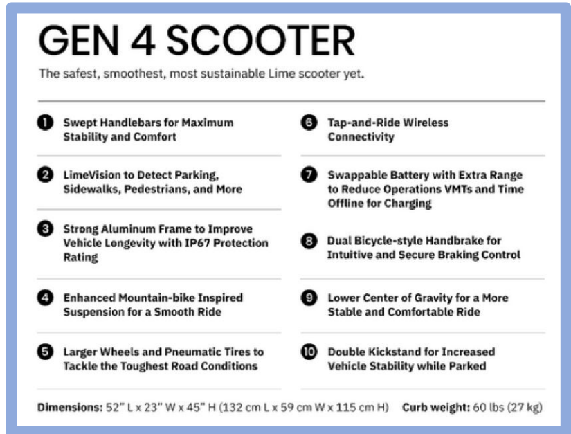
Figure 18 – Lime’s Gen 4 E-scooter Specifications
