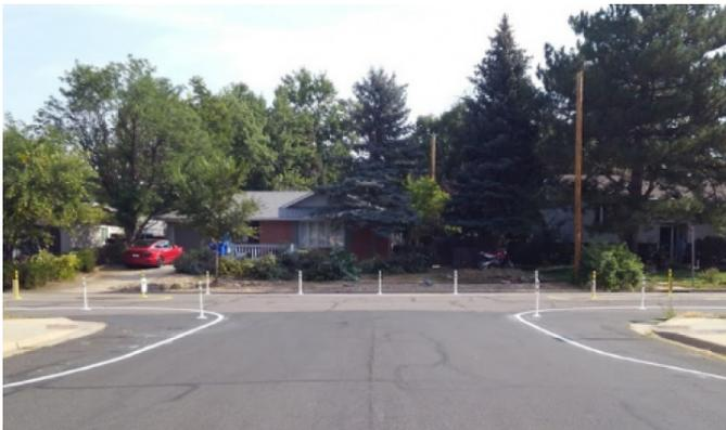
*Figure 9. Median Island and Curb Extensions on Mohawk Drive at Inca Parkway*
