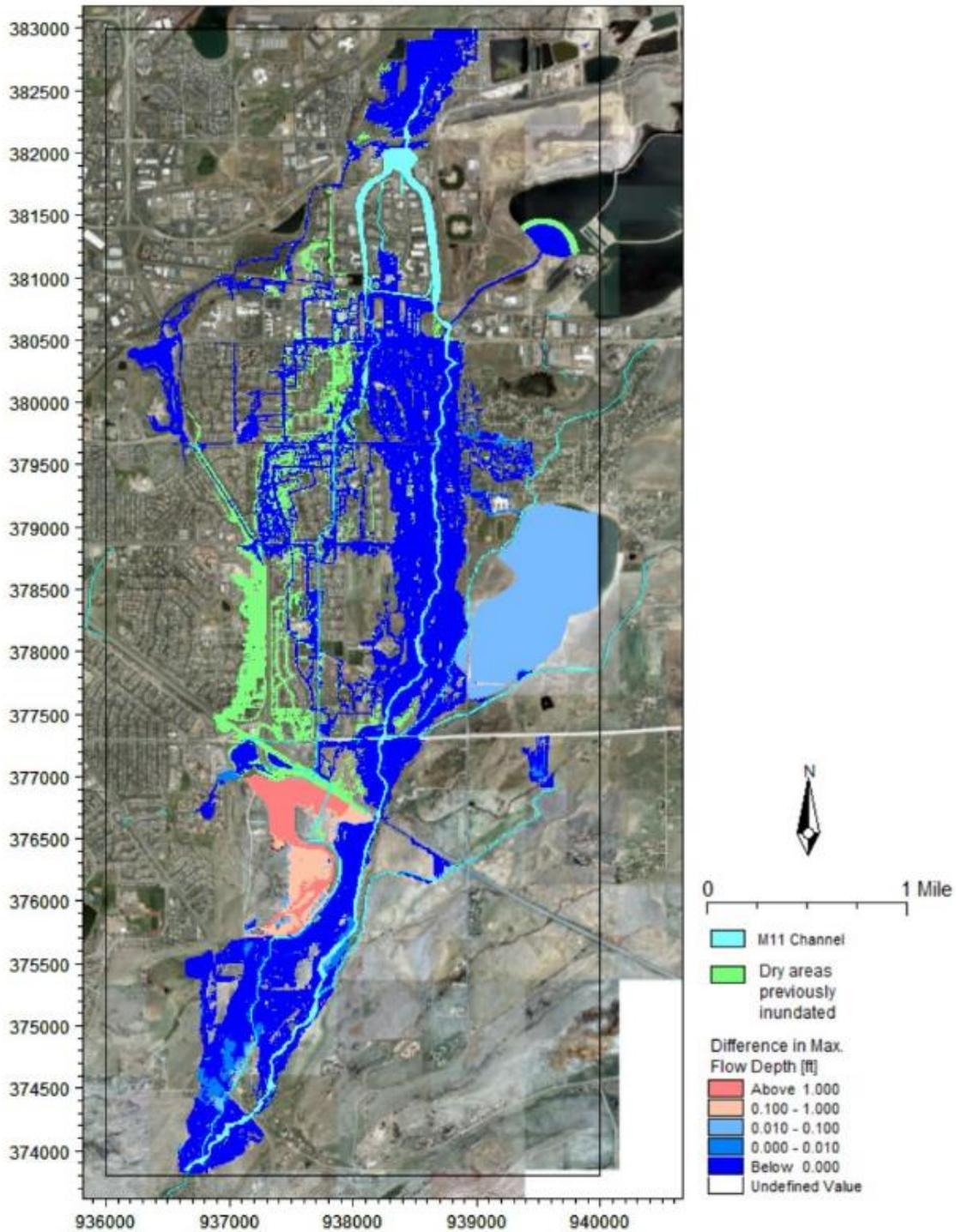
**Figure 9.1:** Difference in 100-year Flood Depth between Corrected Effective Model and Proposed Conditions Model
