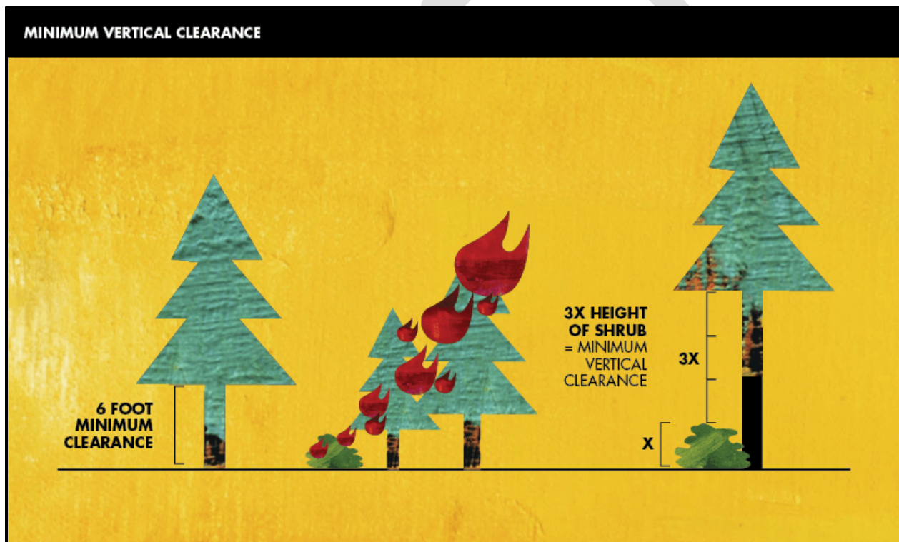
Figure E.3. Recommended minimal vertical clearance.
