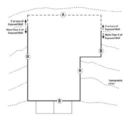
\*Wall area  $\boldsymbol{A}$  is partially exposed above grade by three feet or less. Wall area  $\boldsymbol{B}$  is exposed above grade by more than three feet.
