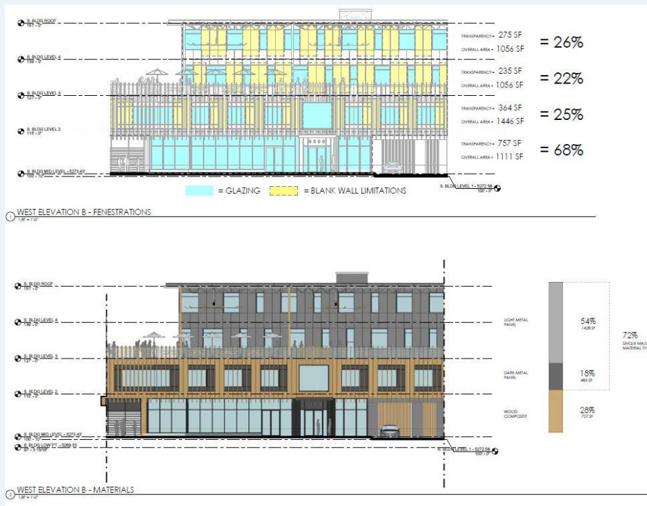
Figure 1: Example of fenestration pattern per floor, and percentage and type of materials
