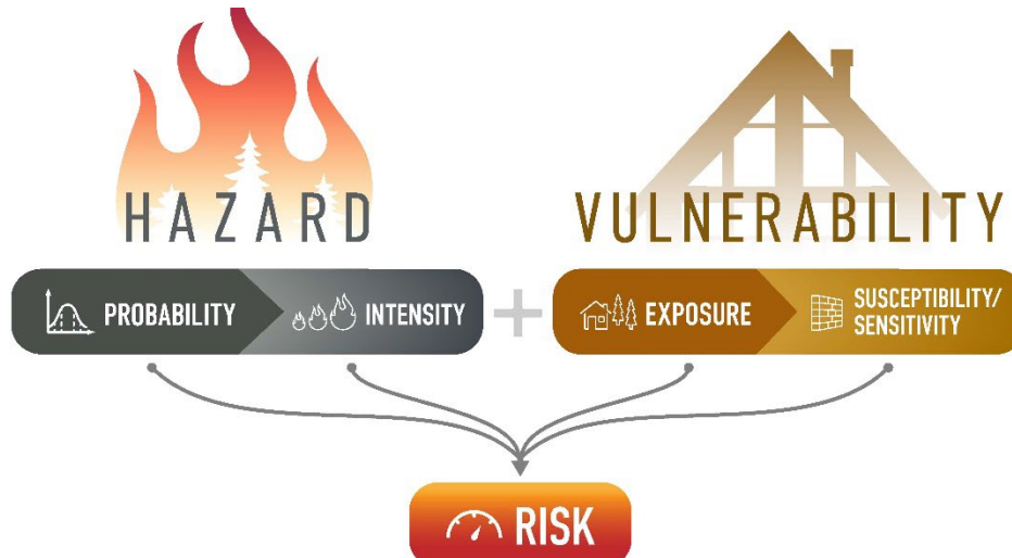
Figure 3.6. Pyrologix’s Quantitative Wildfire Risk Framework for the COAL Quantitative Risk Assessment, derived from Scott et al. (2013).
