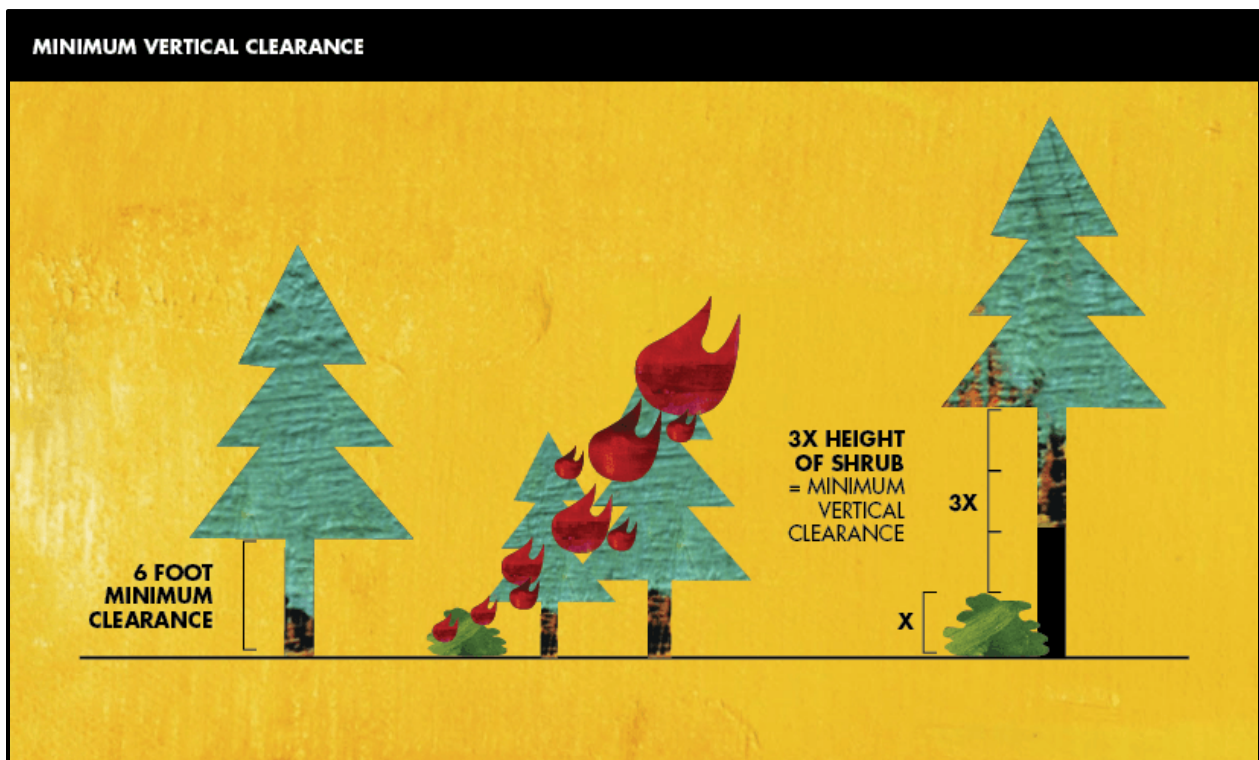
Figure E.3. Recommended minimal vertical clearance.
