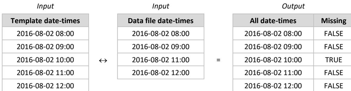
Figure 4. Join process to combine original time-stamp data from the trail counter to a template list of date-times to create a continuous dataset and identify any periods of missing records.
