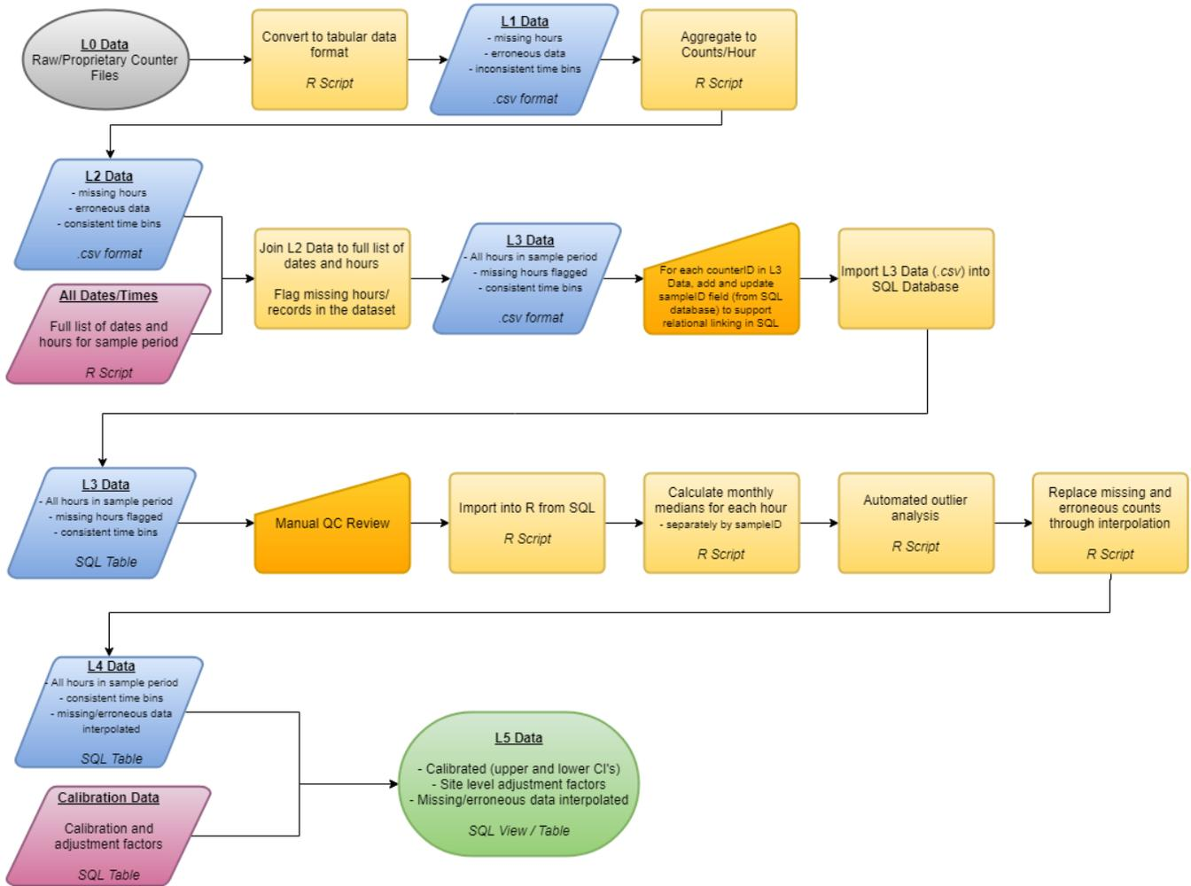
Figure 3. Flow chart of trail counter data processing from Level 0 (raw) to Level 5 (final) data products
