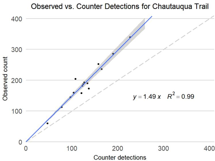
Figure 5. Regression plot showing the relationship between observed counts (y) and counter detections (x) for the Chautauqua Trail sample location. Dashed line represents a theoretical perfect detection rate of 1:1.
