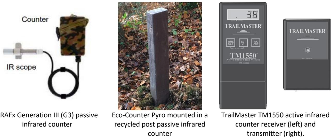
Figure 2. Passive and active infrared trail counters used on city-managed open space.
