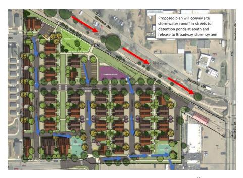
Figure 38 - Stormwater Runoff
