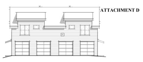
FOURPLEX BBCC - NORTH ELEVATION ELEVATION 1/16" = 1'-0"
