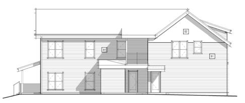
FOURPLEX BBCC - EAST ELEVATION ELEVATION 1/16" = 1'-0"
