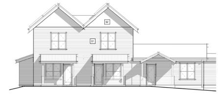
TRIPLEX BBC - SOUTH ELEVATION ELEVATION 1/16" = 1'-0"
