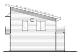
CARRIAGE HOUSE A2- WEST ELEVATION ELEVATION 1/16" = 1'-0"
