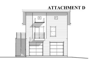
CARRIAGE HOUSE A2- NORTH ELEVATION ELEVATION 1/16" = 1'-0"
