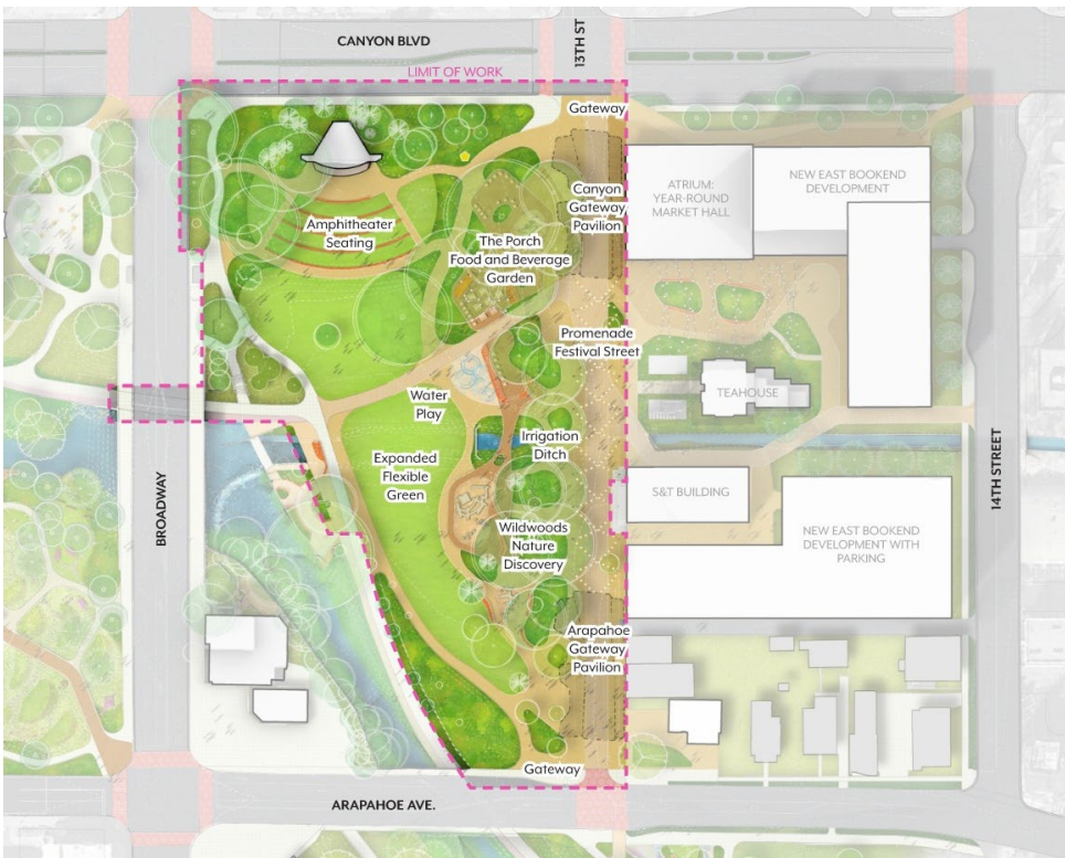
Figure 3: Final Schematic Design: Detailed site plan of the East End illustrating festival street, expanded flexible green space, gateway pavilions, water play area, nature discovery zone, and connections to surrounding streets and park features.
