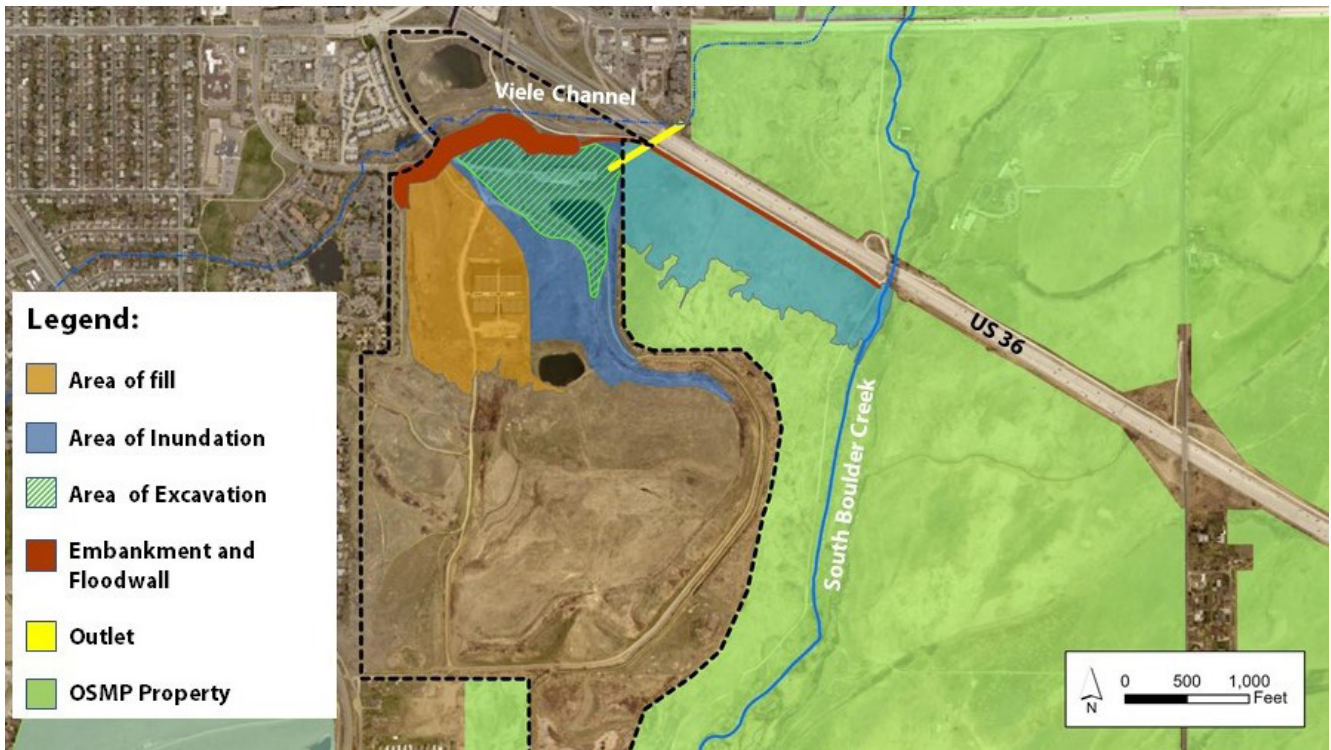
Figure 1: South Boulder Creek Flood mitigation project.
