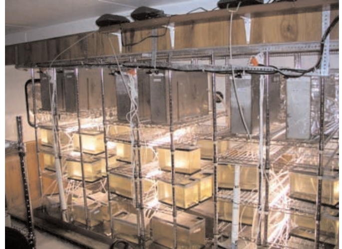
Fish Exposure Mobile Aquaria Aquaria inside the research trailer used by CU and USGS to evaluate impacts of Endocrine Disrupting Compounds.
