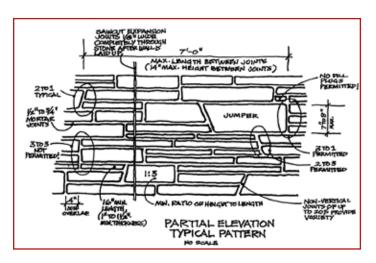
Masons perched on building scaffolds work from a graphic sketch serving as a recipe of how to lay a standard campus sandstone wall.
