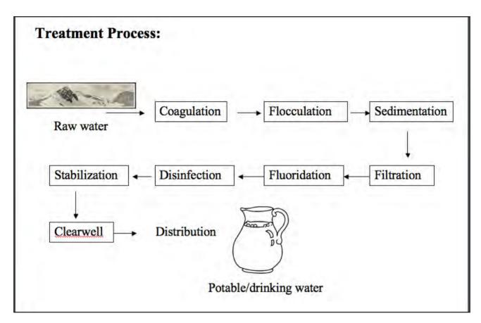
Boulder's water is treated to protect public health, comply with drinking water regulations and standards, and for aesthetic reasons. The current process at the Betasso Water Treatment Plant is graphically depicted in the above diagram.
