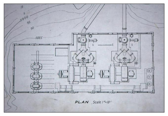
This drawing of the original two generators is a detail from the Central Colorado Power Company's original "Power House and Pressure Line" plan. *Courtesy City of Boulder*
