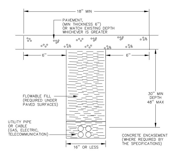
NOTE: IF TRENCH WIDTH IS WIDER THAN 16" USE UTILITY TRENCH DRAWING NO. 4.02
