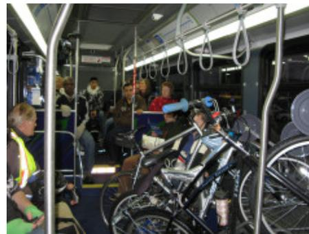
SWIFT BRT service (Seattle, WA) provides on-board storage for 3 bikes in addition to racks on the front of the bus.
