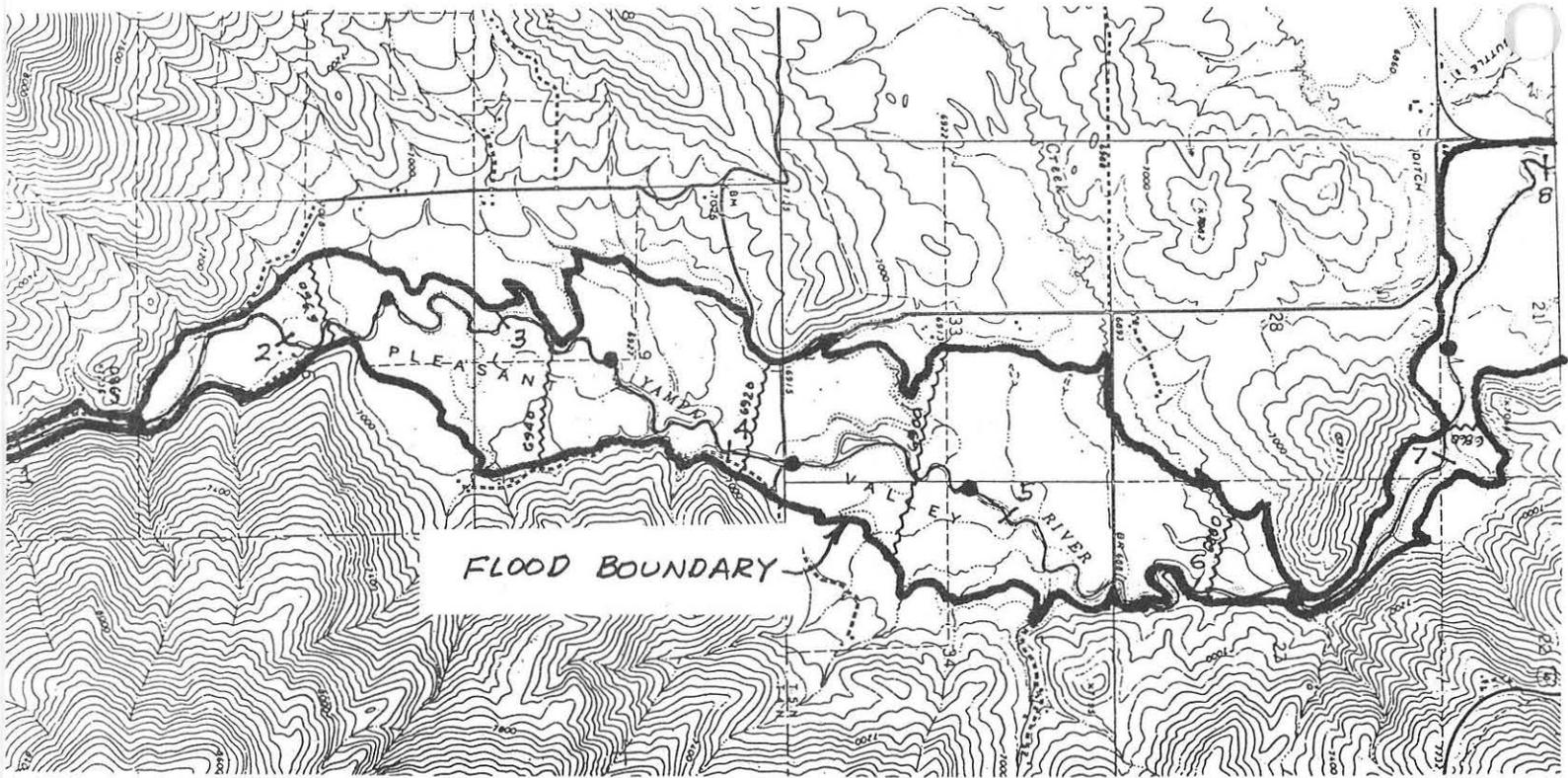
Step 7: Draw flood boundaries with a pencil line by connecting the end points of the flood contours. Flood boundaries should approach ground contours at a tangent and can only cross them at the ends of a flood contour.
