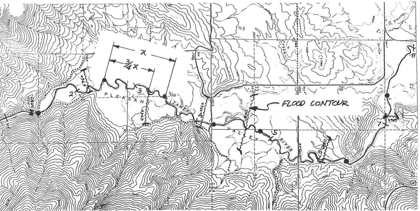
Step 6: For the desired depth (15 feet in this example), interpolate horizontally between points where the ground contours cross the stream (horizontal scaling ratio =  $15/20 = 3/4$  of horizontal distance between ground contours) and mark the location of flood contours in the channel. In this example, if "x" is the distance between points where ground contours cross the channel then the flood contours shall cross the channel at about  $3/4$  of the distance "x" from the upstream point.
