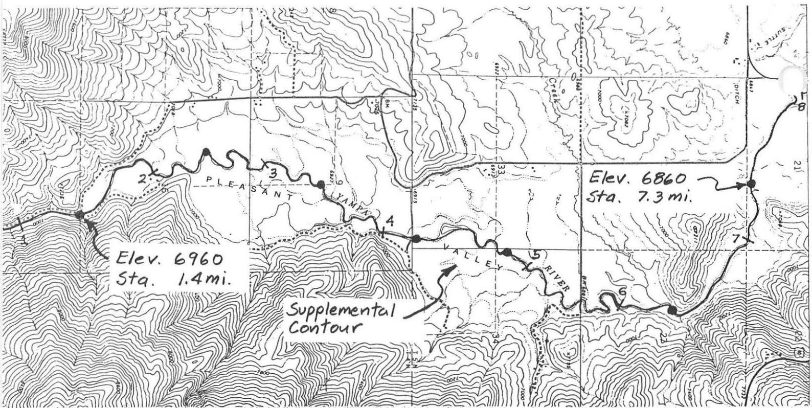
Step 2: Mark where the ground contours cross the stream centerline. Note that while the contour interval for the map is 40 feet, supplemental contours have been shown in the vicinity of the river as dashed lines so the actual available contour interval is 20 feet for this reach.
