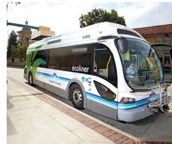
Foothill Transit's "Ecoliner" coaches run on electricity without overhead wires. Find out more about the Proterra Ecoliner [here](#).
