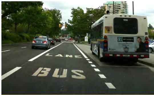
This curbside bus lane on Marine Drive in Vancouver, BC includes a priority signal and queue jump that allows buses to bypass traffic queued to cross the Lions Gate Bridge; buses carry about a quarter of peak-hour traffic on the bridge.
