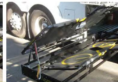
For intercity commuter buses the inclusion of a SportWorks luggage bay carrier racks allows for three bicycles to be stored securely and out of inclement weather. These racks are currently available on AC Transit's Interbay buses in Alameda and Contra Costa counties.
