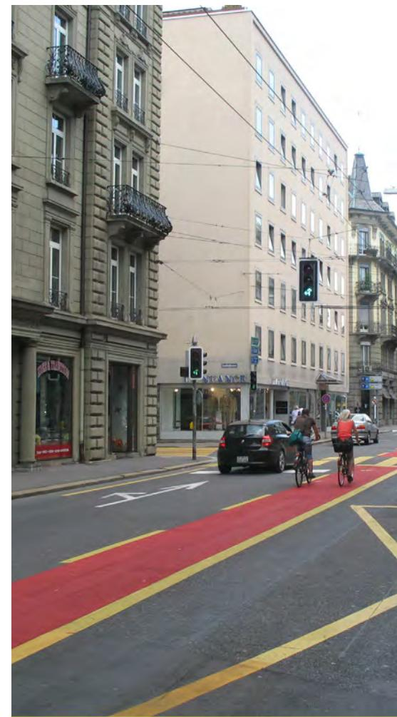
A painted bicycle lane separates this bus lane in Lucerne, Switzerland from general-purpose traffic. Yellow pavement markings within the bus lane provide further delineation.
