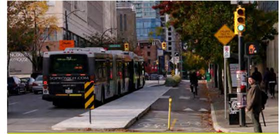
The Dunsmuir Separated Bike Lane in Vancouver BC is an example of a separated cycle track with a sidewalk that is clearly defined from the cycle track, and a bus stop with defined transitions to the sidewalk for safe pedestrian movement.
