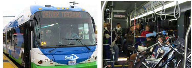
Swift BRT vehicles allow bicycles on board using custom bicycle racks. This extends the catchment of BRT ridership and allows multi-modal commuting for passengers.
