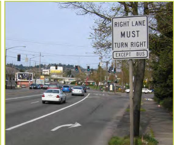
Queue jumps allow buses to bypass traffic to reach a stop at the far side of the intersection (Portland, OR).
