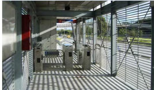
Bogotá, famous for its extensive Transmilenio BRT system, has developed simple station designs that include turnstiles before entry to the station, real time arrival information and announcements, and station attendants.
