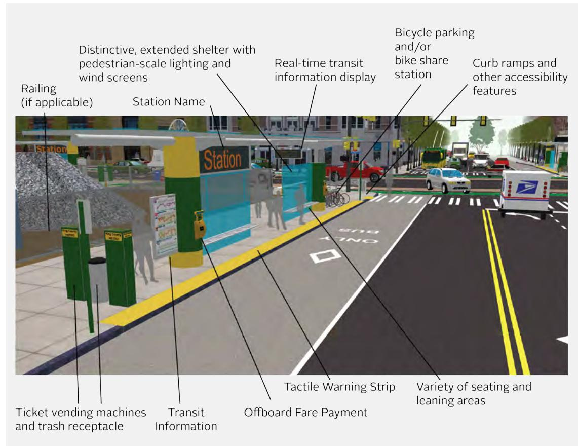
This design illustrates elements of a high amenity transit stop, with features designed to help integrate modes, accommodate the needs of different user types, and provide information and convenience to the passenger.
