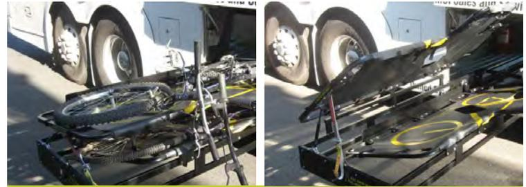
For intercity commuter buses the inclusion of a SportWorks luggage bay carrier racks allows for three bicycles to be stored securely and out of inclement weather. These racks are currently available on AC Transit's Interbay buses in Alameda and Contra Costa counties.
