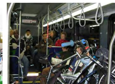
Swift BRT vehicles allow bicycles on board using custom bicycle racks. This extends the catchment of BRT ridership and allows multi-modal commuting for passengers.
