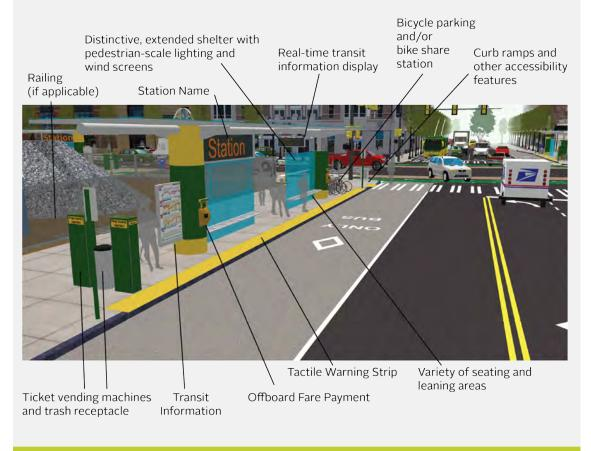
This design illustrates elements of a high amenity transit stop, with features designed to help integrate modes accommodate the needs of different user types, and provide information and convenience to the passenger. Source: Nelson\Nygaard
