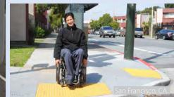
▲ Universal Design: Intersections should provide facilities that can safely move people of all ages and capabilities across the street. Design elements like curb ramps, level landings and gutter seams, visible and audile signals, smooth surfaces, accessible push buttons (or default WALK phases), and signage that may help pedestrians navigate intersections should be integrated into intersection design.
