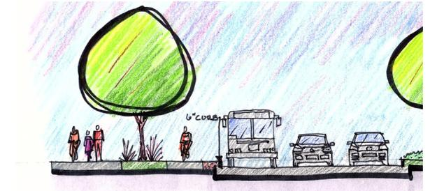
A narrow paved buffer separates the protected bike lane from the roadway, and a wide amenity zone with street trees is located between the protected bike lane and the multi-use path.
