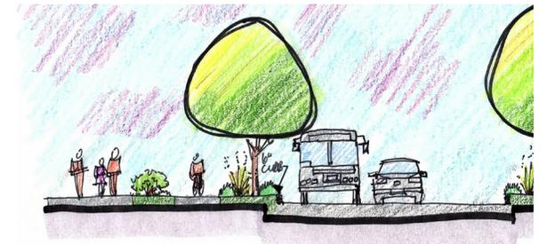
A wide amenity zone with street trees separates the protected bike lane from the roadway, and a narrower amenity zone is located between the protected bike lane and multi-use path.
