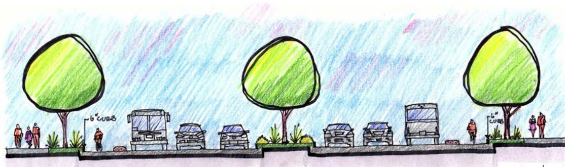
Figure H-6 District C - Alt 3 Side-Running BRT with Raised Protected Bike Lane and Multi-Use Path (C.3.1a)
