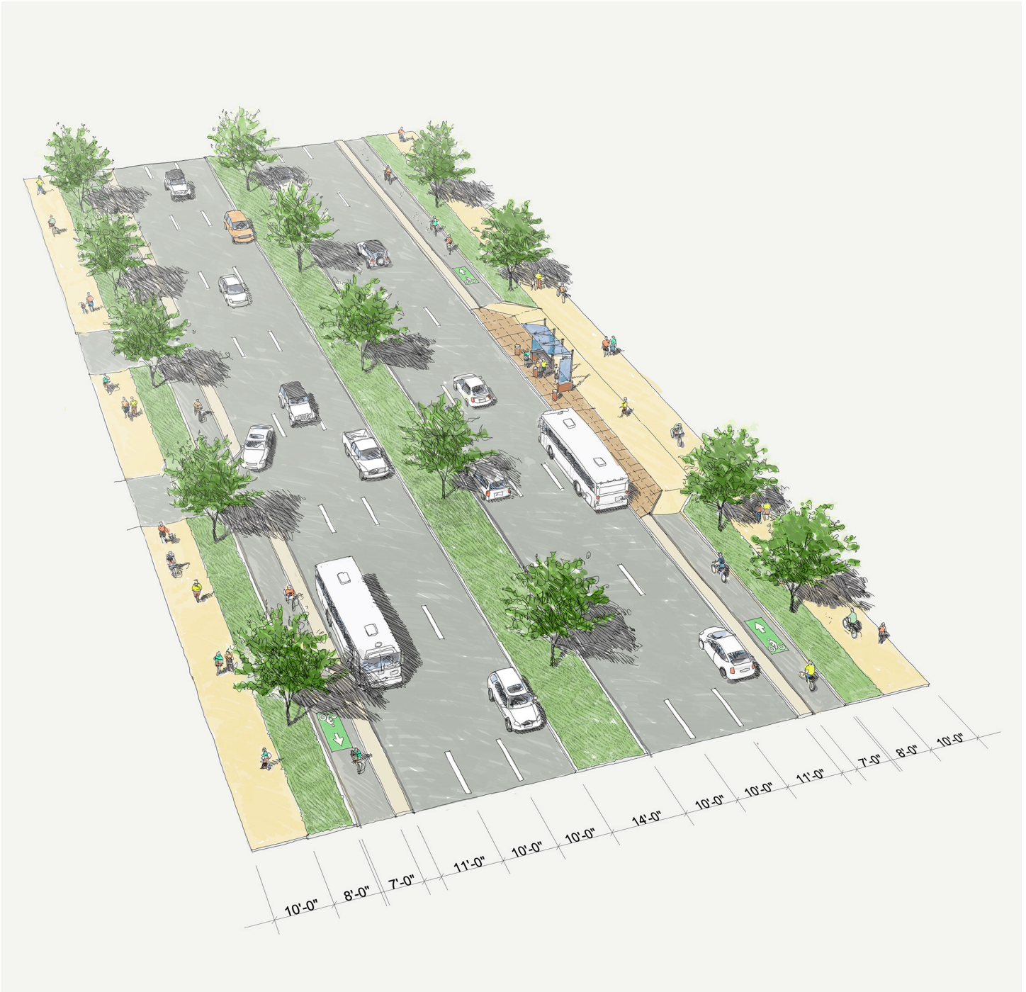
Figure H-5 District C - Alt 2 Enhanced Bus with Street-level Protected Bike Lane and Multi-Use Path (C.2.3)
