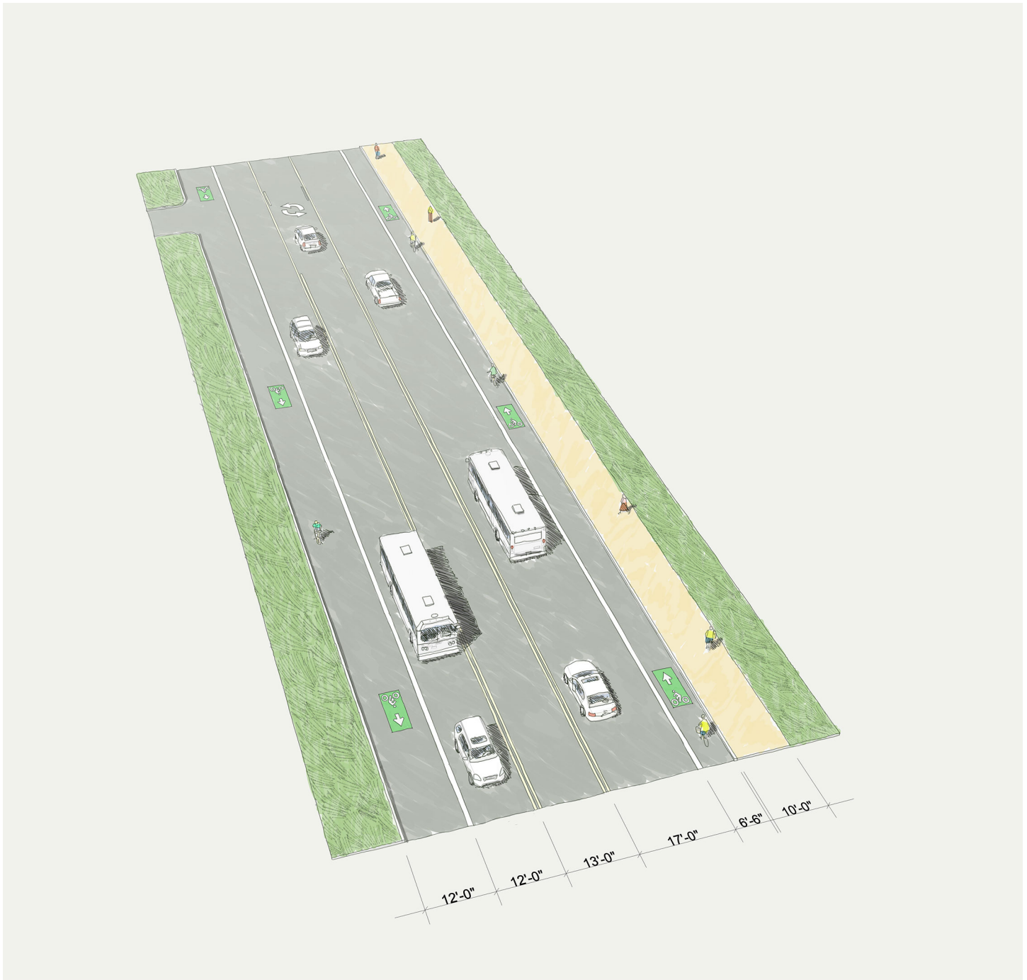
Figure H-10 District E - Alt 2 Enhanced Bus with Street-level Bike Lane and Sidewalk or Multi-Use Path (E.2.4)
