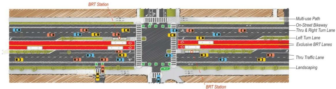
Alternative D: Center-running BRT in an exclusive transit lane with three general purpose lanes, an on-street bikeway, and a completed multi-use path
