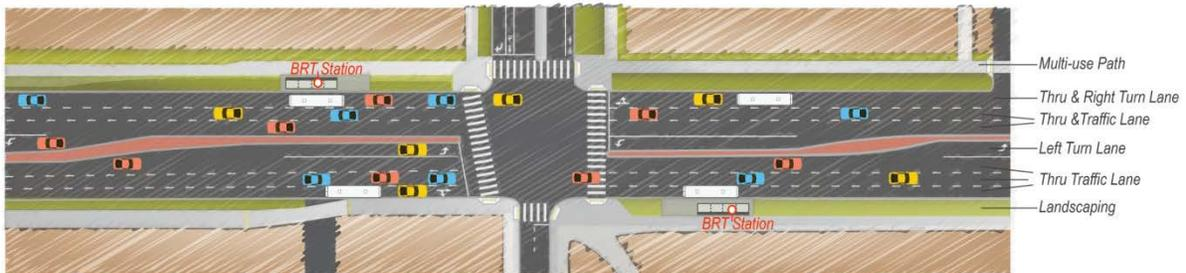
Alternative A: Enhanced bus in mixed-traffic with three general-purpose lanes and a completed multi-use path for pedestrians and bicycles
