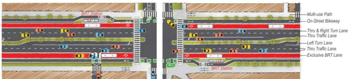
Alternative C: Center-running BRT in an exclusive transit lane with two general purpose lanes, an on-street bikeway, and a completed multi-use path
