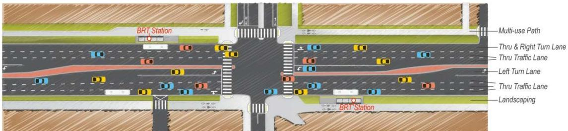
Alternative B: Side-running BRT in a semi-exclusive business-and-transit (BAT) lane (allows right turns) with two general purpose lanes, an on-street bikeway, and a completed multi-use path
