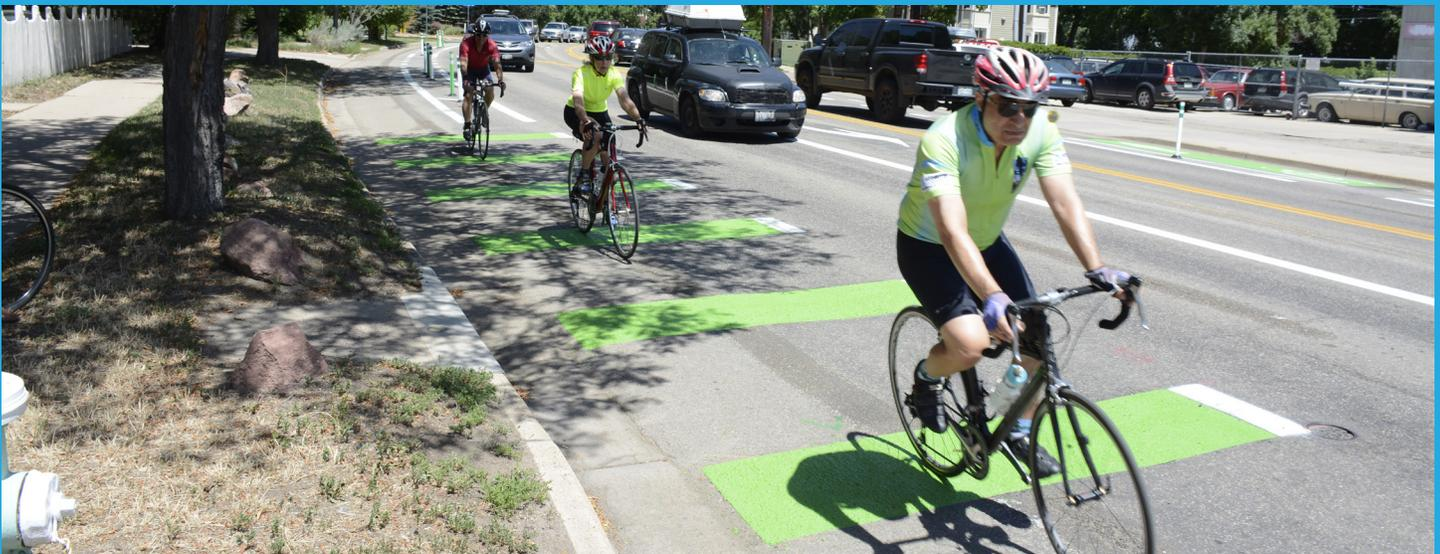
**Green pavement markings:** Green bike lanes were installed on Folsom Street on the northbound approaches at Canyon Boulevard and Pearl Street in September 2012. After the installation, the number of northbound right-hook collisions decreased at both locations. These markings were recently reconfigured as part of the Folsom Street Living Laboratory project. The effectiveness of green markings installed in other locations will continue to be evaluated.
