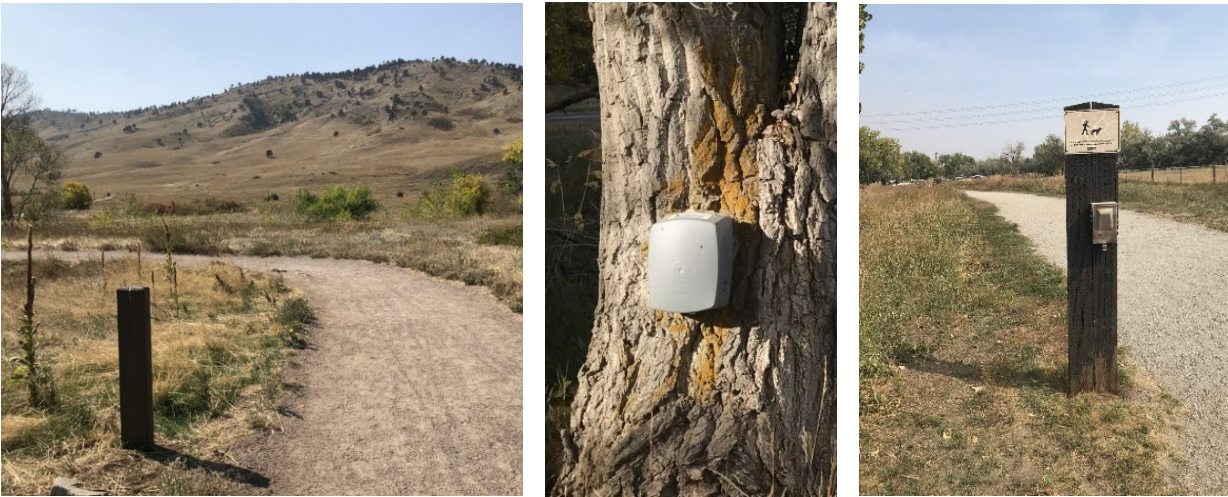
Figure 2. Types of passive infrared trail counters used in the study. From left to right: Eco-Counter PYRO, Eco-Counter PYRO-Box, TRAFx Generation III.
