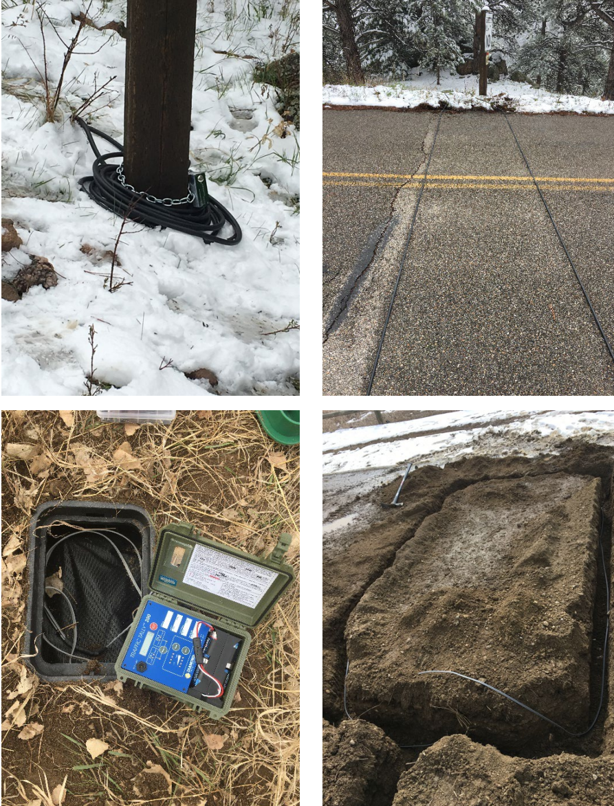
Figure 1. Types of vehicle counters used in the study. Top row: Diamond Traffic Products Road Runner 3 with pneumatic road tubes. Bottom row: Diamond Traffic Products Traffic Tally 200™ with inductive loops.
