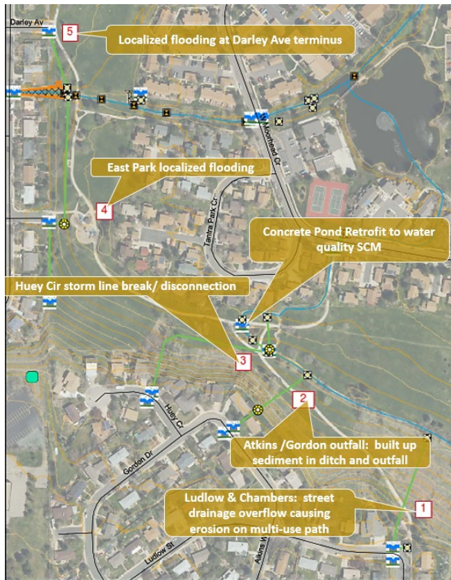
Figure 6. Tantra Park Documented Drainage Issues
