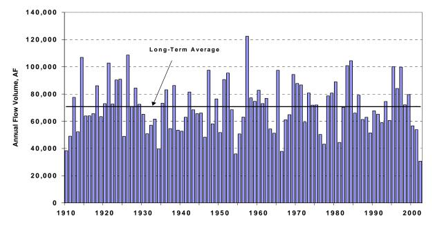
FIGURE 5-30. NATURAL FLOW FOR BOULDER CREEK NEAR ORODELL RECONSTRUCTED FROM GAGE RECORDS<sup>143</sup>
