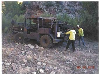
Photograph 1: ATV Tire Drill Rig.
