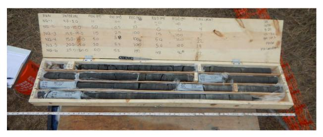
Photograph 13: B-211(P); Core box 1 of 1 [Pierre Shale]
