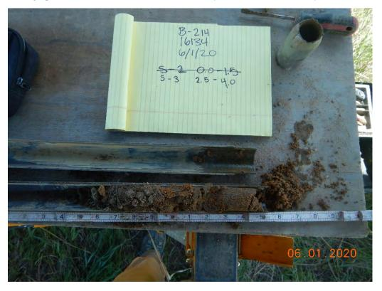
Photograph 12: B-214(P); S-3 from 2.5 to 4.0: Poorly Graded Sand with Silt and Gravel [Alluvium]
