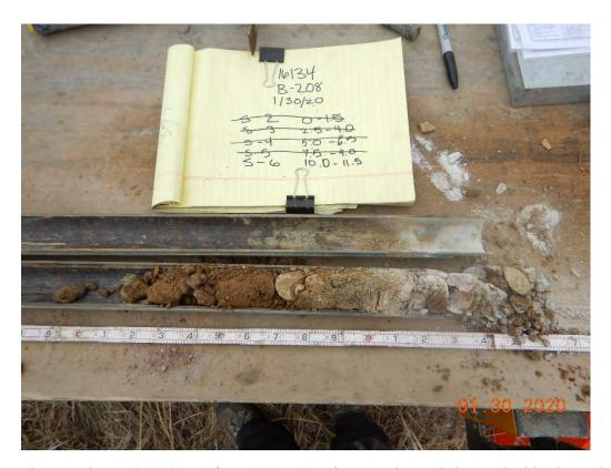
Photograph 7: B-208(P); S-6 from 10.0 to 11.5 feet: Poorly Graded Gravel with Clay and Sand [Alluvium]
