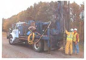
Photograph 3 - Truck Mounted Drill Rig
