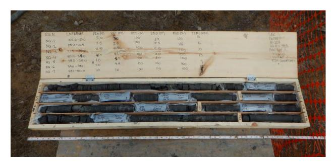
Photograph 4: B-204(P); Core box 1 of 1 [Pierre Shale]
