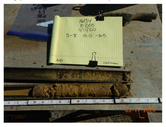
Photograph 4: B-205(P); S-8 from 15.0 to 16.5 feet: Poorly Graded Gravel with Clay and Sand [Alluvium]
