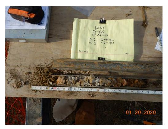
Photograph 9: B-210; S-3 from 2.5 to 4.0 feet: Clayey Gravel with Sand [Fill]
