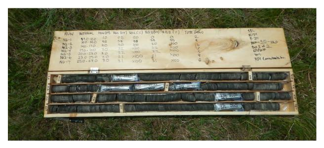
Photograph 16: B-214(P); Core box 1 of 3 [Pierre Shale]
