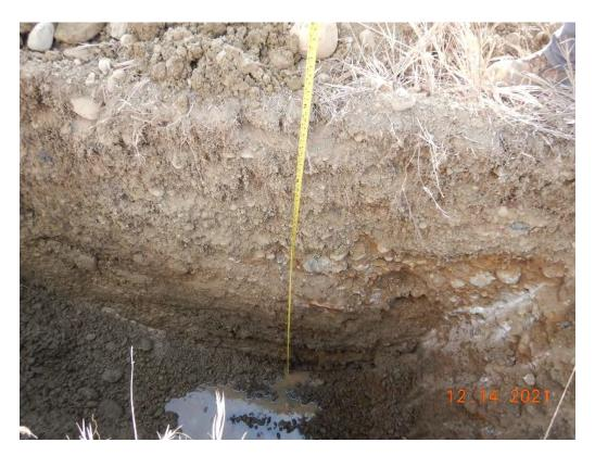
Photograph 21: TP-205 fill from 0.0 to 5.5 feet, and Pierre Shale from 5.5 to 7.0 feet.
