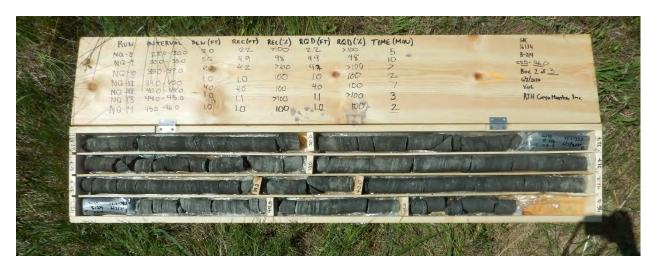
Photograph 17: B-214(P); Core box 2 of 3 [Pierre Shale]
