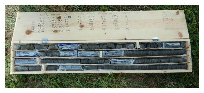
Photograph 19: B-215(P); Core box 1 of 3 [Pierre Shale]
