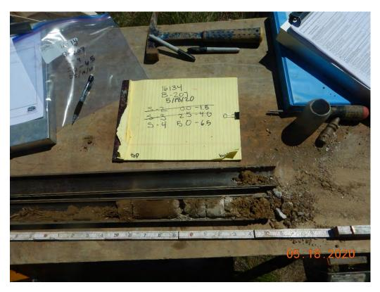
Photograph 5: B-207(P); S-4 from 5.0 to 6.5 feet: Poorly Graded Sand with Silt and Gravel [Alluvium]
