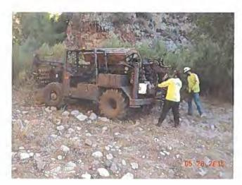
Photograph 4 – ATV Tire Drill Rig
