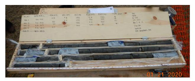
Photograph 11: B-210; Core box 1 of 2 [Pierre Shale]
