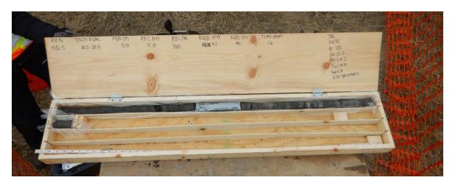
Photograph 12: B-210; Core box 2 of 2 [Pierre Shale]
