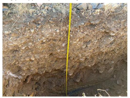
Photograph 12: TP-203 fill from 0.0 to 7.0 and Pierre Shale from 7.0 to 9.5 feet.
