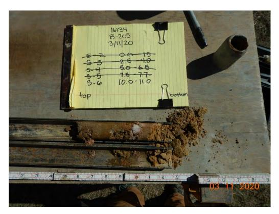
Photograph 3: B-205(P); S-6 from 10.0 to 11.0 feet: Poorly Graded Sand with Silt and Gravel [Alluvium]
