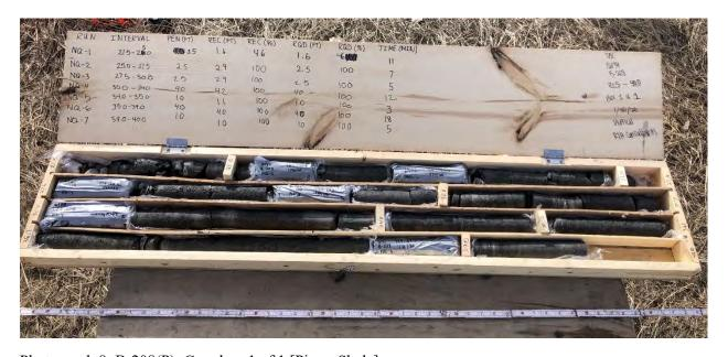
Photograph 8: B-208(P); Core box 1 of 1 [Pierre Shale]
