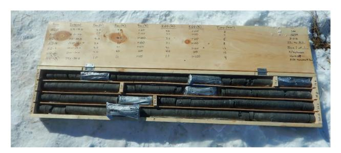
Photograph 14: B-212(P); Core box 1 of 1 [Pierre Shale]
