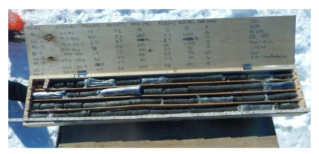
Photograph 3: B-203(P); Core box 1 of 1 [Pierre Shale]
