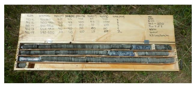
Photograph 18: B-214(P); Core box 3 of 3 [Pierre Shale]
