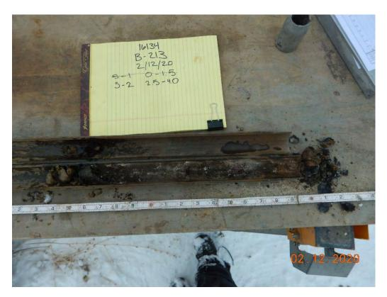
Photograph 11: B-213; S-2 from 2.5 to 4.0: Poorly Graded Sand with Clay and Gravel [Fill]
