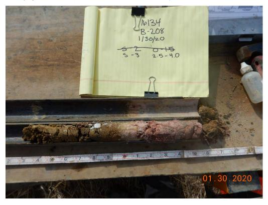
Photograph 6: B-208(P); S-3 from 2.5 to 4.0 feet: Clayey Sand with Gravel [Fill]
