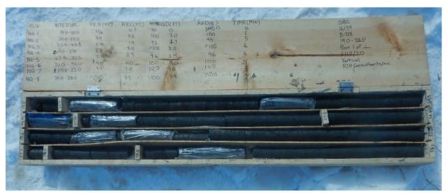
Photograph 1: B-201(P); Core box 1 of 1 [Pierre Shale]
