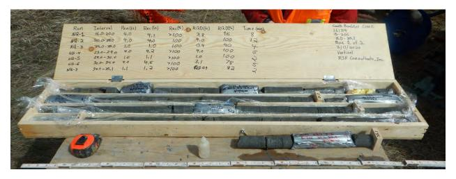
Photograph 6: B-206; Core box 1 of 1 [Pierre Shale]
