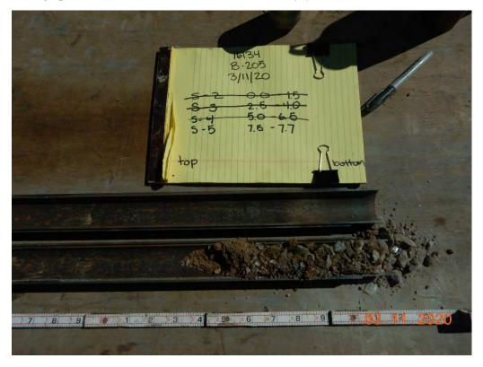
Photograph 2: B-205(P); S-5 from 7.5 to 7.7 feet: Poorly Graded Sand with Silt and Gravel [Alluvium]
