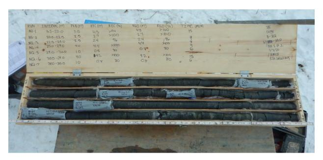
Photograph 2: B-202(P); Core box 1 of 1 [Pierre Shale]
