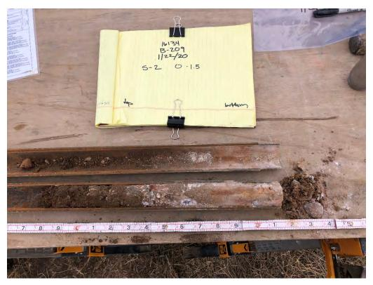
Photograph 8: B-209(P); S-2 from 0.0 to 1.5 feet: Poorly Graded Gravel with Clay and Sand [Fill]
