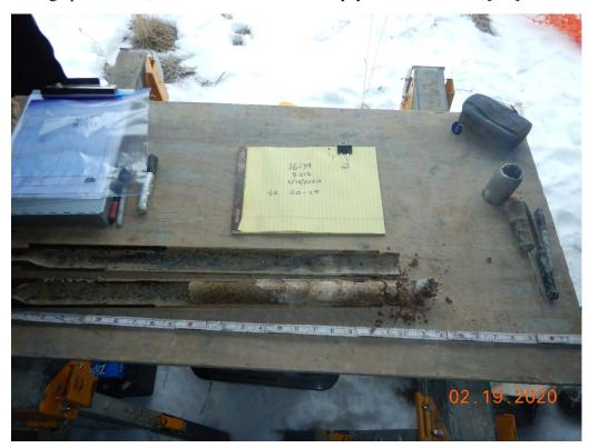
Photograph 10: B-212(P); S-2 from 0.0 to 1.5 feet: Silty Sand with Gravel [Fill]
