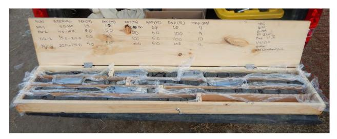
Photograph 9: B-209(P); Core box 1 of 2 [Pierre Shale]
