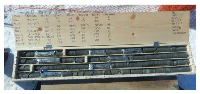
Photograph 15: B-213; Core box 1 of 1 [Pierre Shale]
