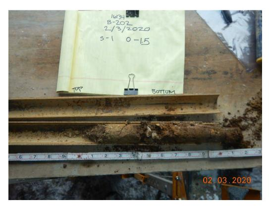
Photograph 1: B-201(P); S-1 from 0.0 to 1.5 feet: Clayey Sand with Gravel [Fill]
