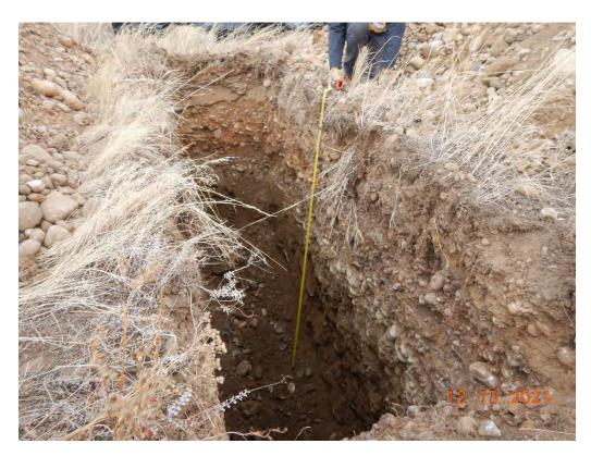
Photograph 3: TP-201 alluvium from 0.0 to 9.0 feet.
