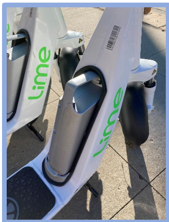
Figure 17 – Lime's Swappable Battery
