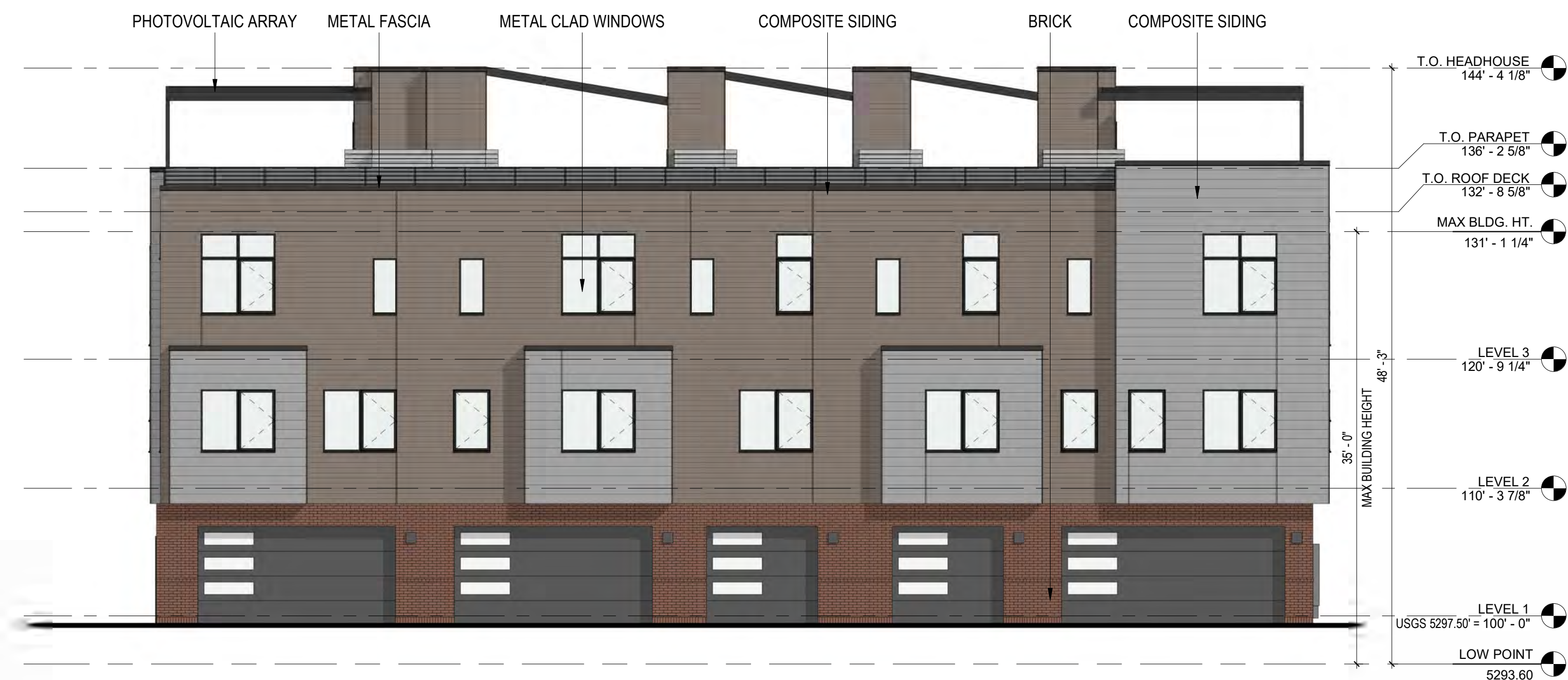
BUILDING 3 - WEST ELEVATION 1/8" = 1'-0"
