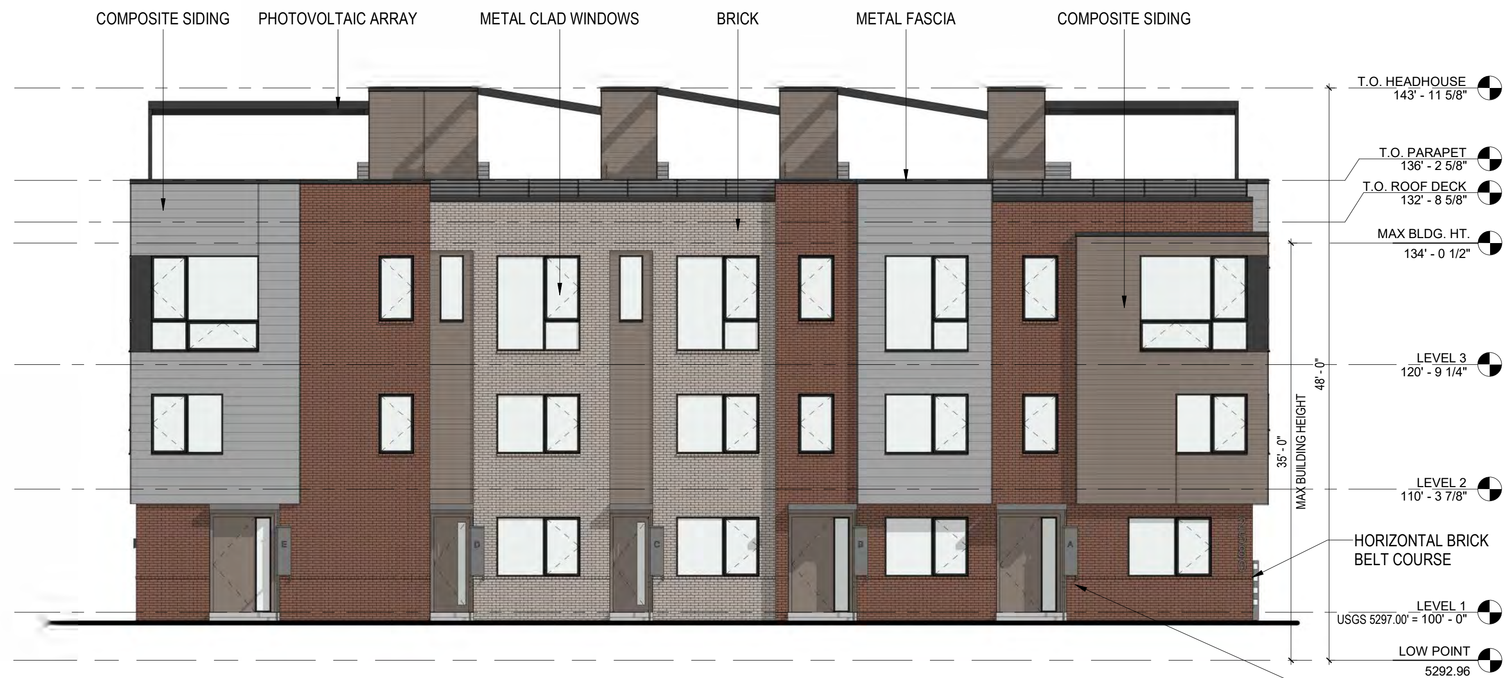
BUILDING 2 - WEST ELEVATION
