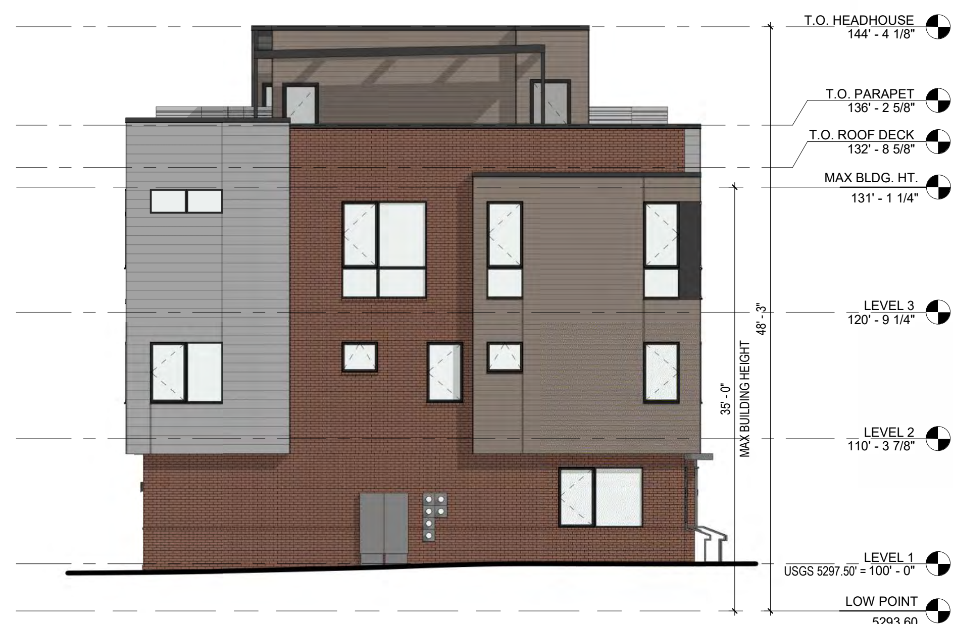
BUILDING 3 - SOUTH ELEVATION 1/8" = 1'-0"
