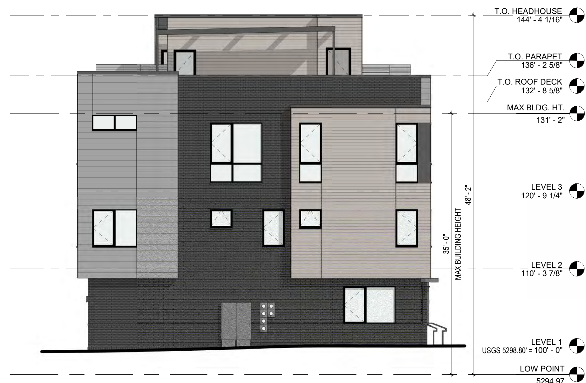
BUILDING 6 - SOUTH ELEVATION
