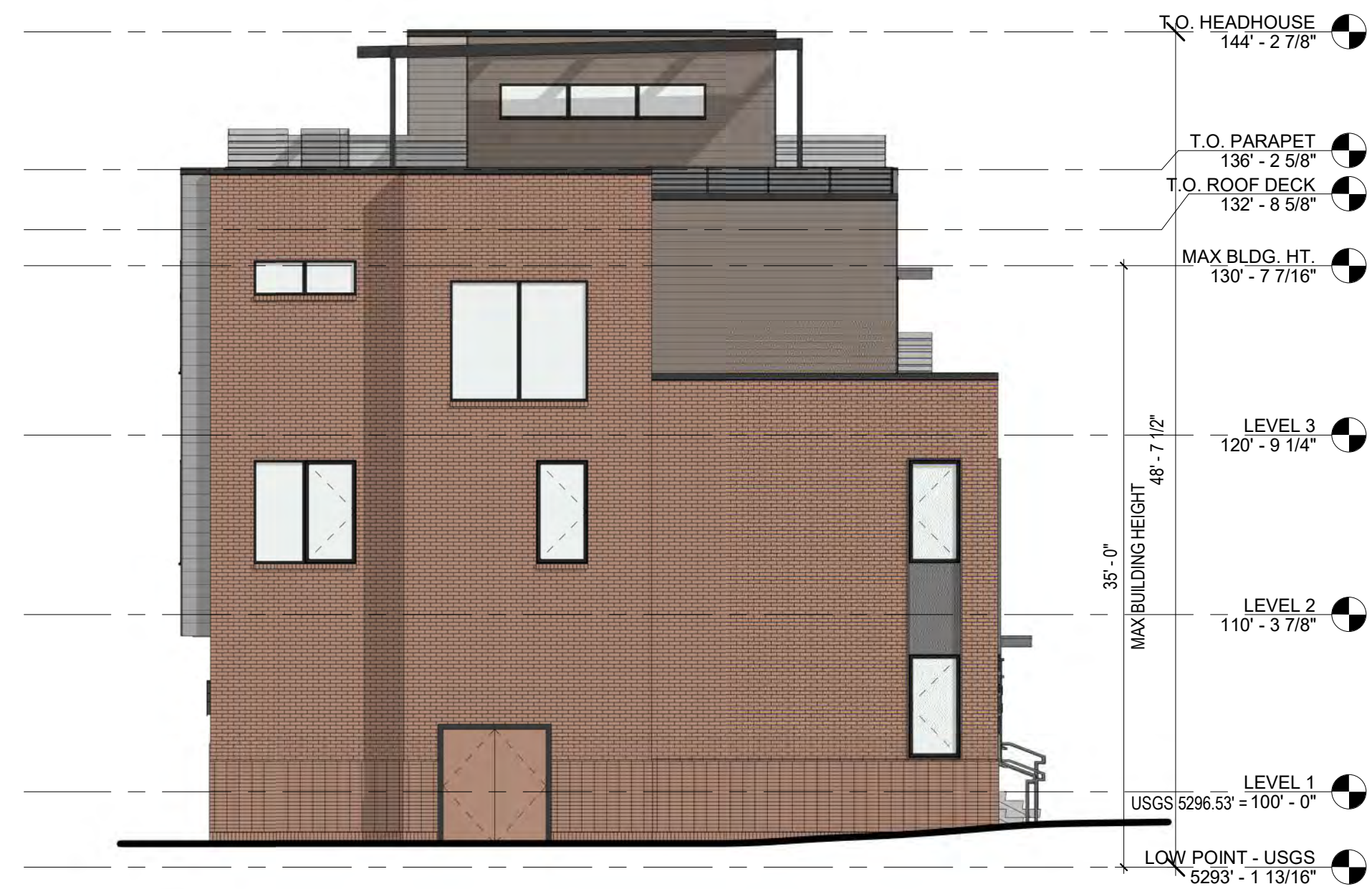
BUILDING 5 - EAST ELEVATION
