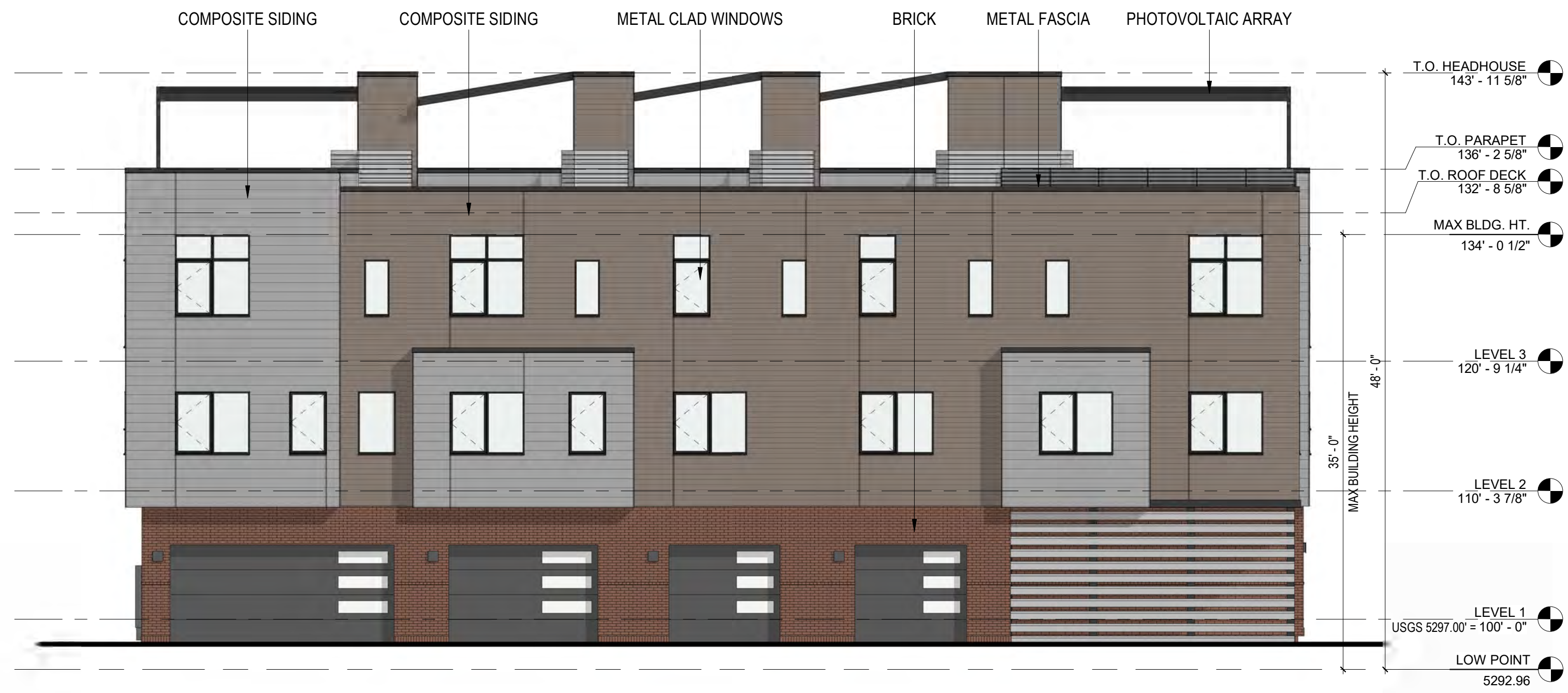
BUILDING 2 - EAST ELEVATION
