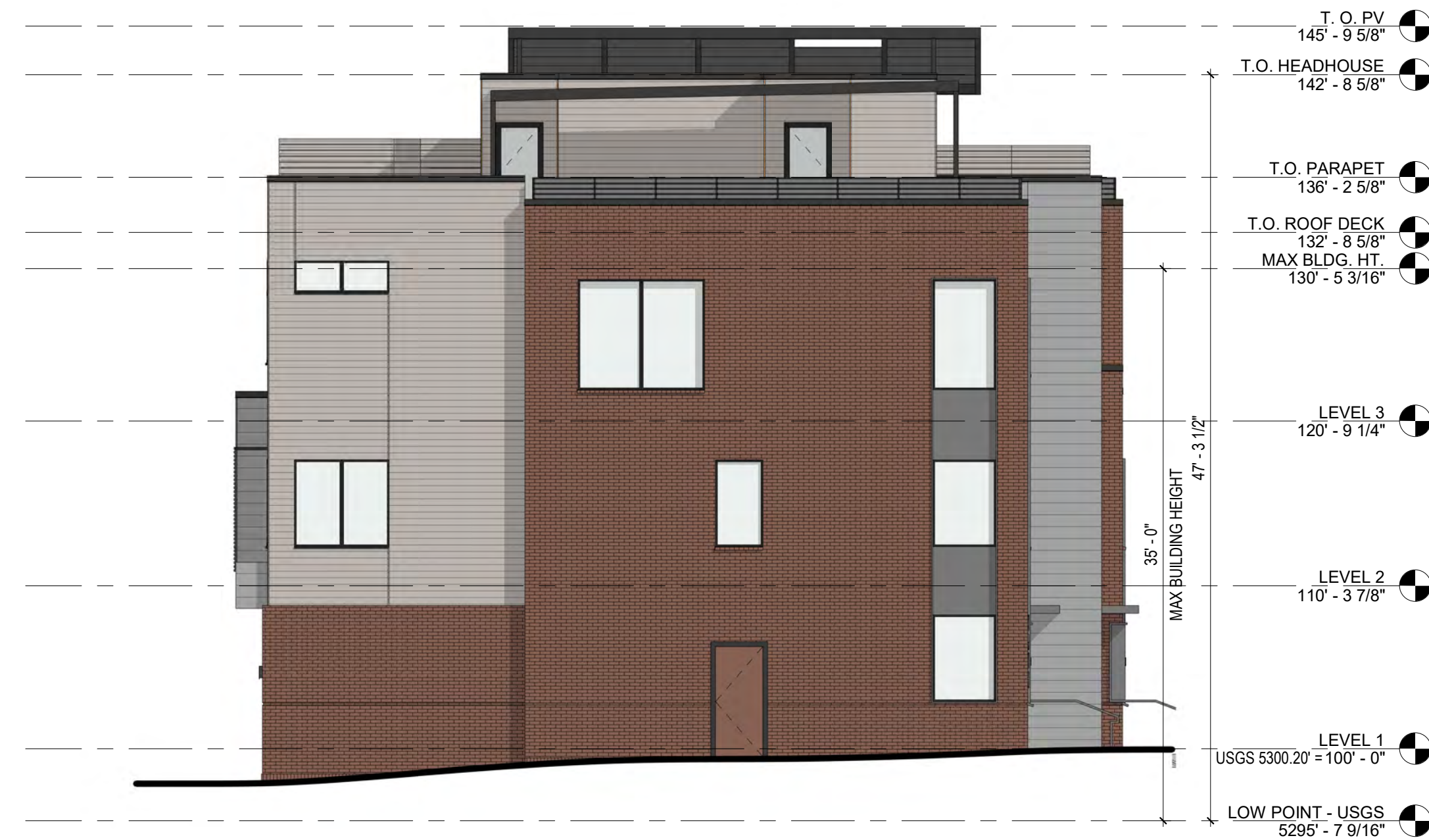
4 BUILDING 7 - NORTH ELEVATION 1/8" = 1'-0"
