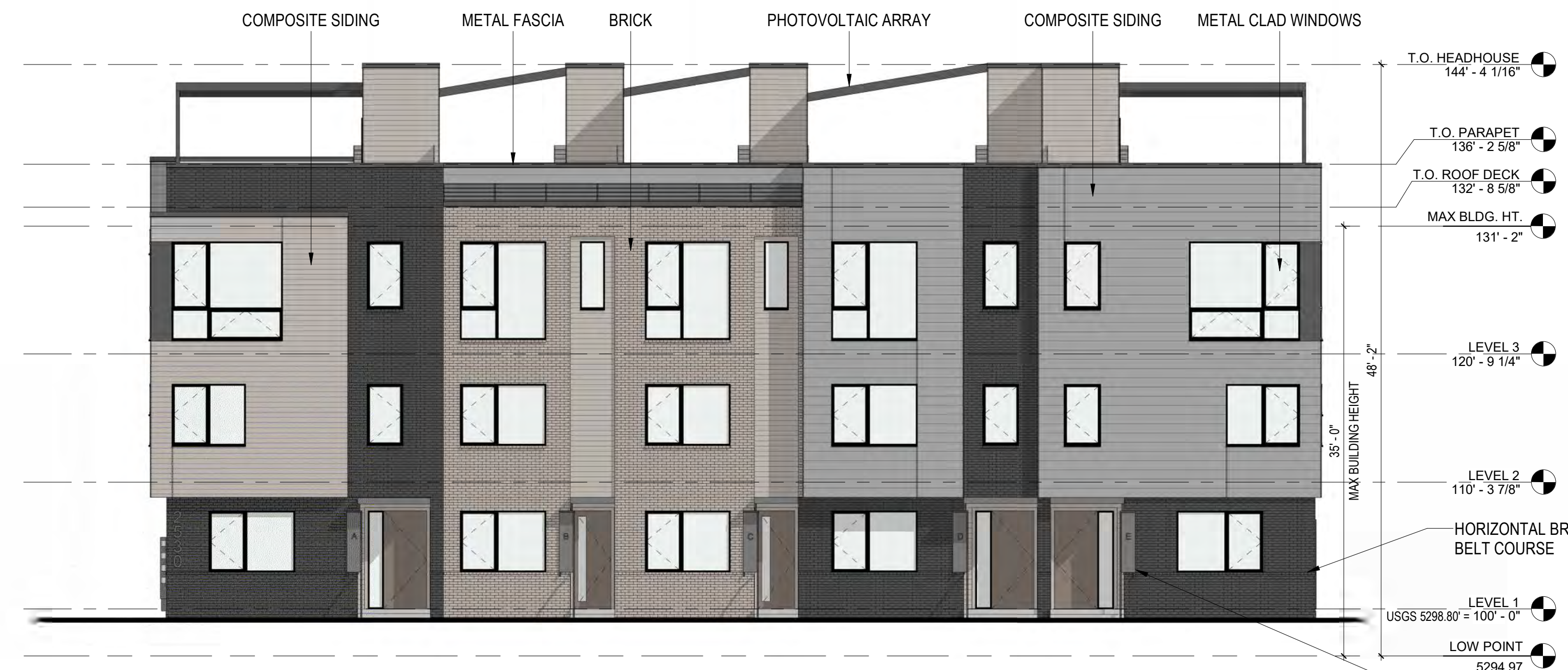
BUILDING 6 - EAST ELEVATION
