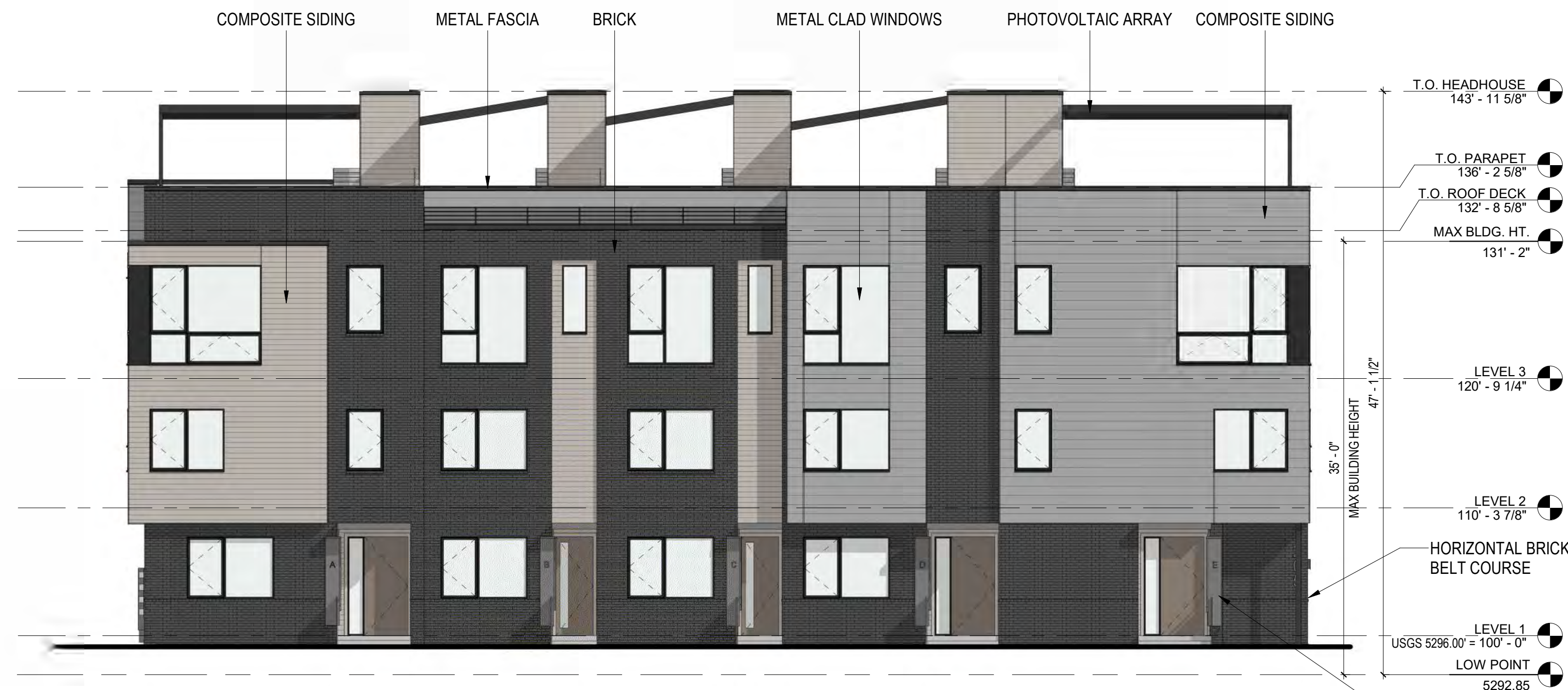
BUILDING 1 - EAST ELEVATION
