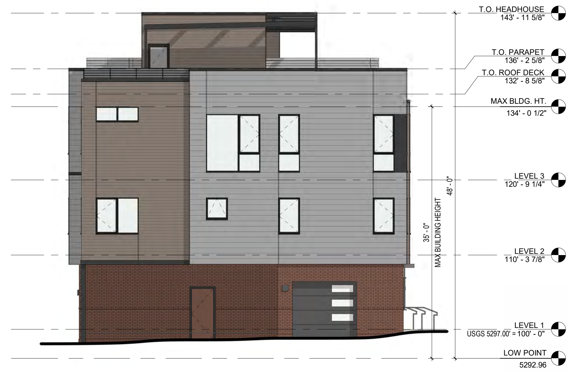
BUILDING 2 - NORTH ELEVATION
