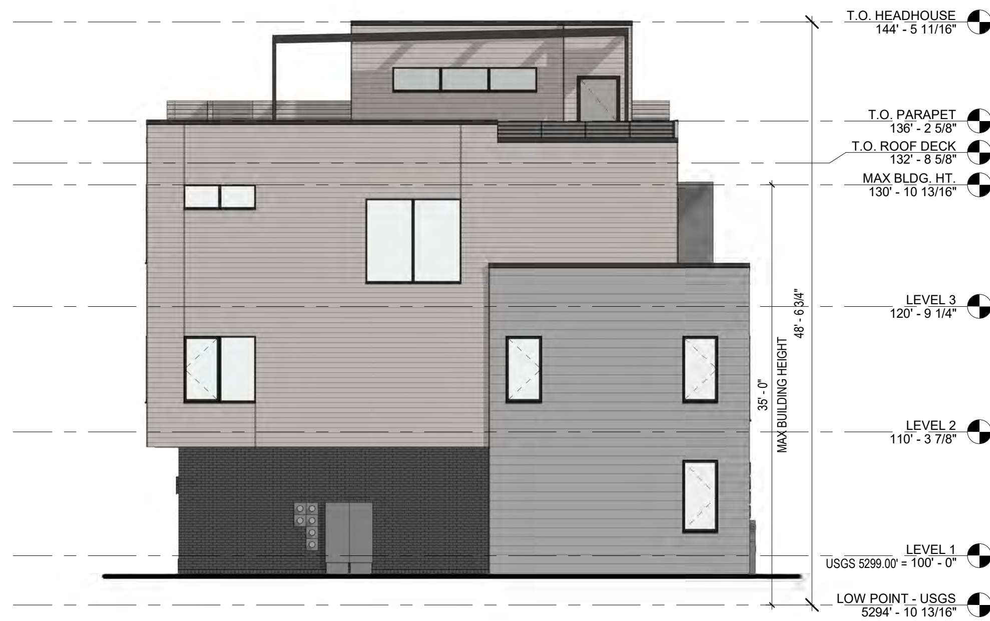
BUILDING 8 - EAST ELEVATION
