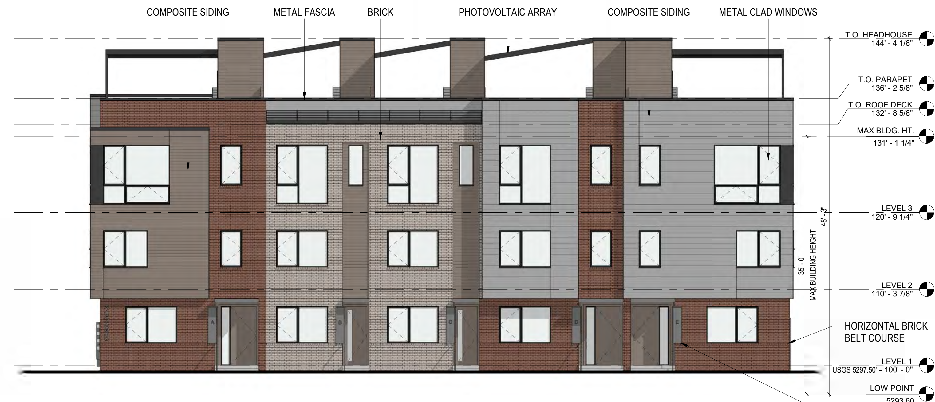
BUILDING 3 - EAST ELEVATION 1/8" = 1'-0"
