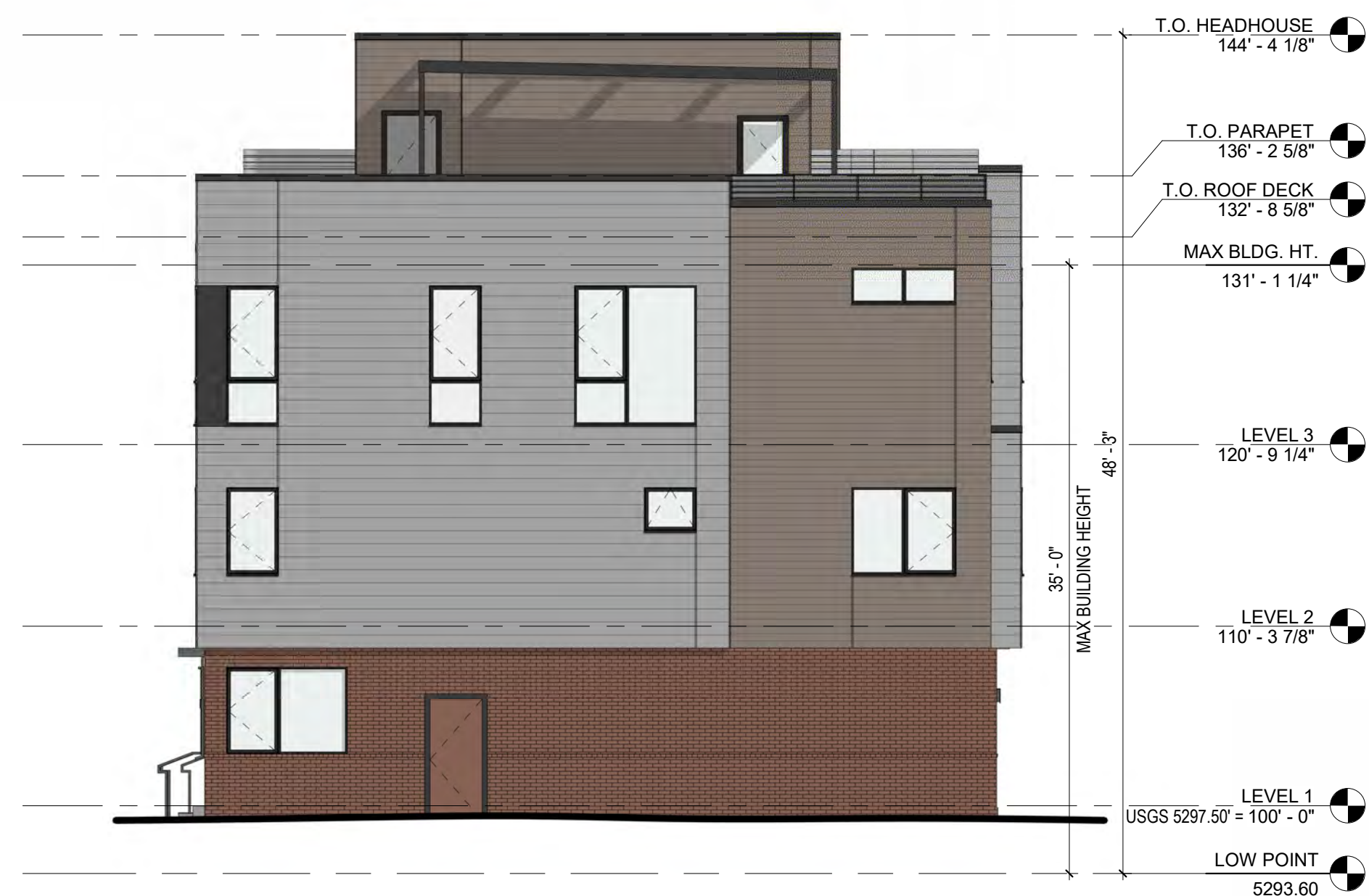
BUILDING 3 - NORTH ELEVATION 1/8" = 1'-0"
