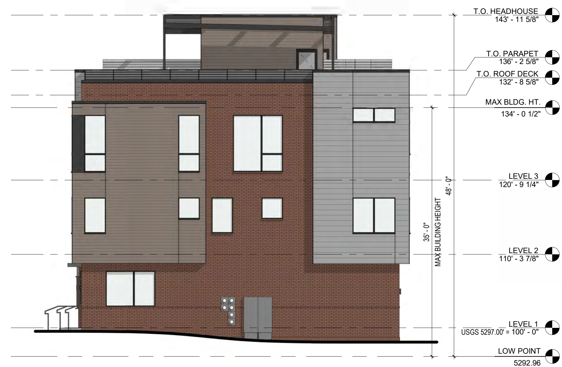
BUILDING 2 - SOUTH ELEVATION
