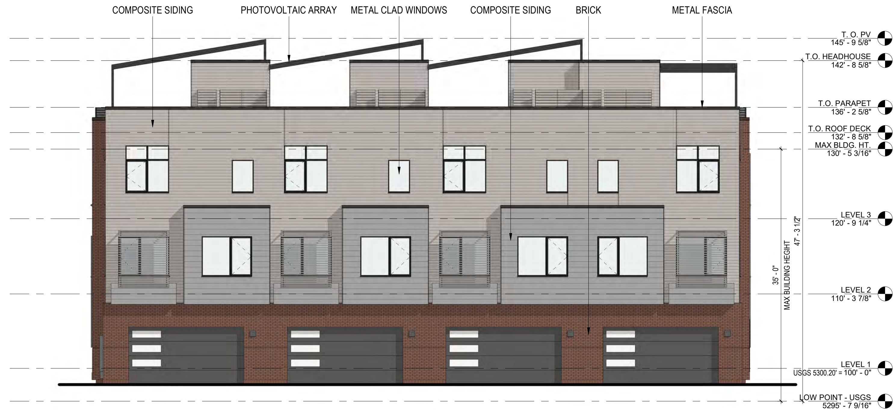
2 BUILDING 7 - EAST ELEVATION 1/8" = 1'-0"
