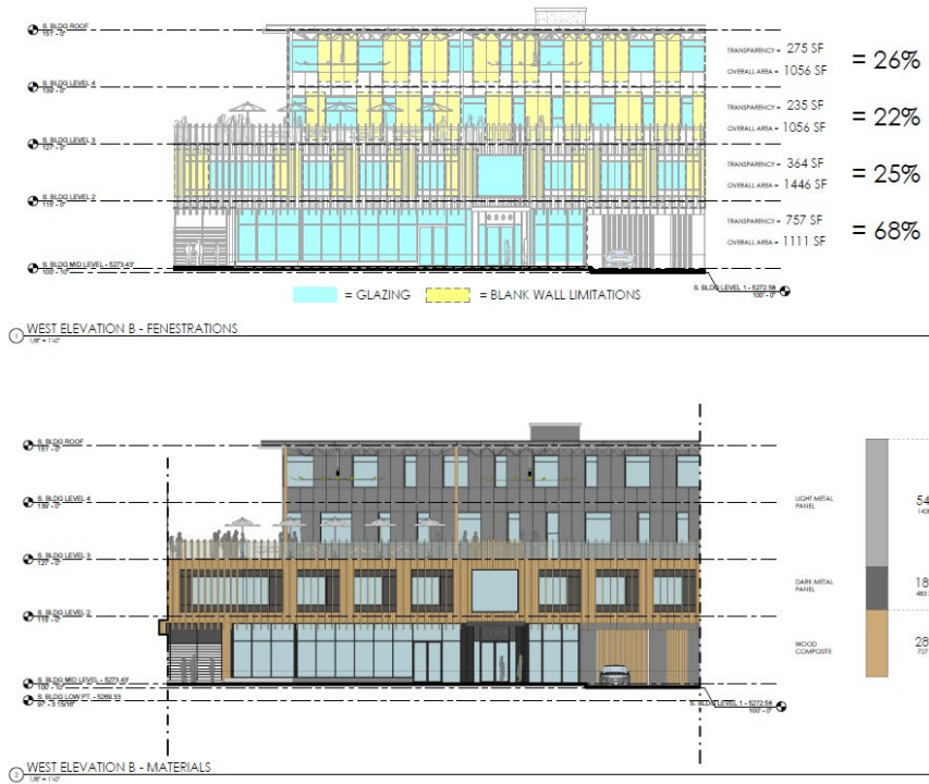
Figure 1: Example of fenestration pattern per floor, and percentage and type of materials
